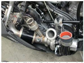
1. Install the TiAL muffler by placing the end of the muffler into the tunnel exhaust reinforcement plate and aligning the muffler to the TiAL exhaust housing on the turbo.
