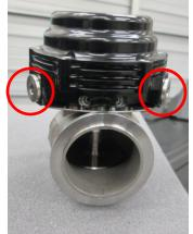
5. Plug the two bottom air holes on the front of the TiAL wastegate. Be sure to use Loctite.
