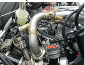
3. Install the turbo inlet between the exhaust housing and the exhaust pipe using the stock donut. Install a V-band clamp between the exhaust housing and the turbo inlet.
