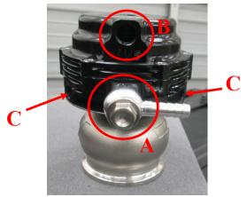
6. Install a banjo fitting using Loctite into the lower air hole on the back of the TiAL wastegate (A). Leave the upper air hole open (B). Leave the two water inlet ports open (C).
