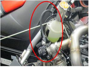
8. Install the black hose between the banjo fitting on the TiAL wastegate and the perpendicular barb on the boost solenoid. Your TiAL exhaust system is now installed.
