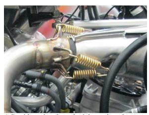
4. Double spring the turbo inlet to the exhaust pipe.
