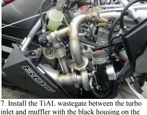
inlet and muffler with the black housing on the wastegate facing to the left. Secure the waste gate using the small V-band clamps.
