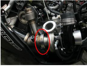
2. Install a V-band clamp between the exhaust housing and the muffler. Align the clamp so that the bolt is on the bottom.
