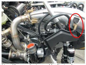
Note: If you are having trouble aligning the turbo inlet with the exhaust pipe, remove the spring in the center of the exhaust pipe, install the inlet, and then reinstall the spring.
