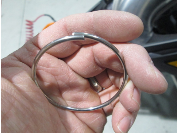
1. Bend throttle body lock rings slightly until the ends overlap.
