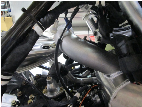
5. Start the air box into place. Make sure the throttle cable is on the left hand side of the inlet tube.
