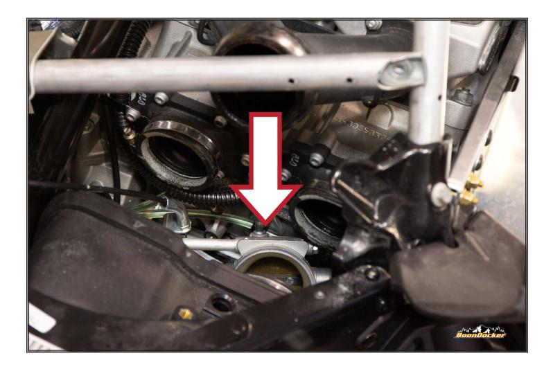
Unbolt throttle body and push down out of the way.
