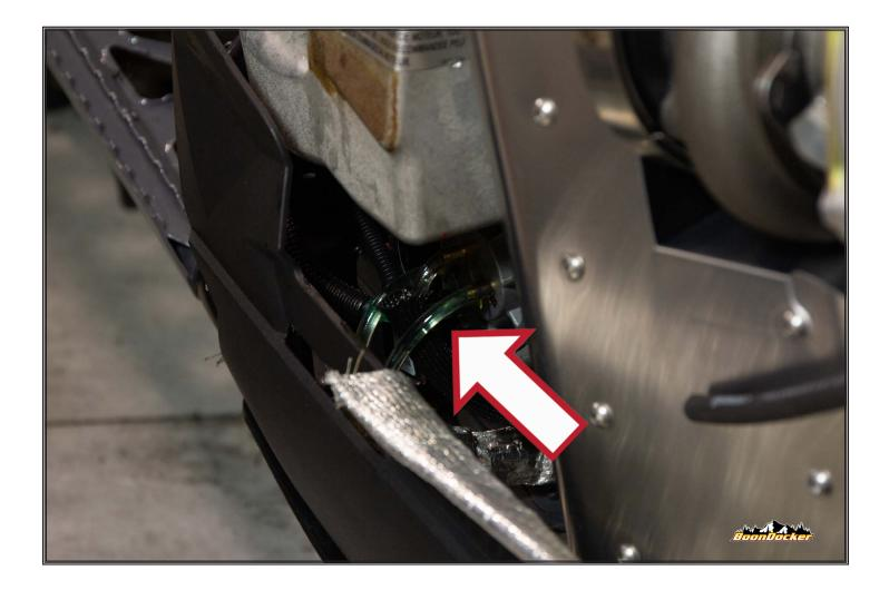
2020+ Model only: Remove previously unhooked oil line from oil pump, purge and install BoonDocker oil line onto pump and secure with 4" zip tie.
