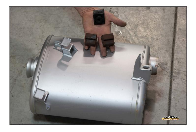
Remove rubber grommets from stock mufflrer.
