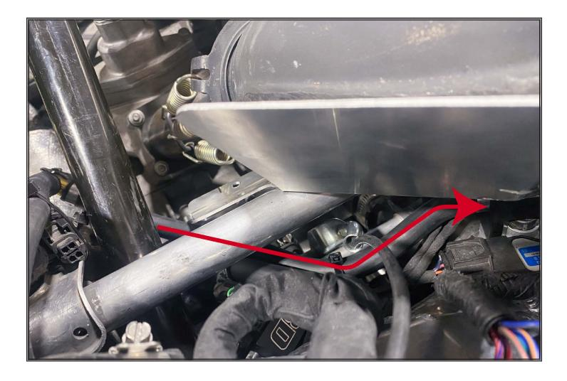
Route PTO fuel line to auxillary injector as shown. Take special care to ensure the line does not kink.
