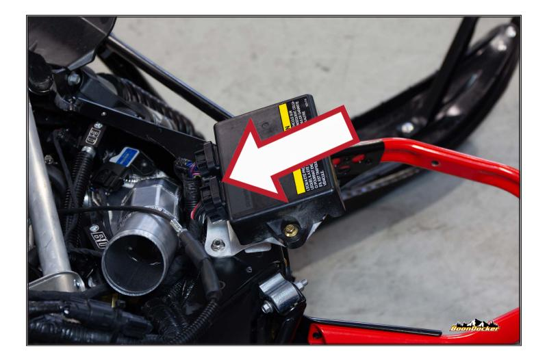
Install ECU relocate bracket and re-install ECU. Plug control box into ECU as shown.
