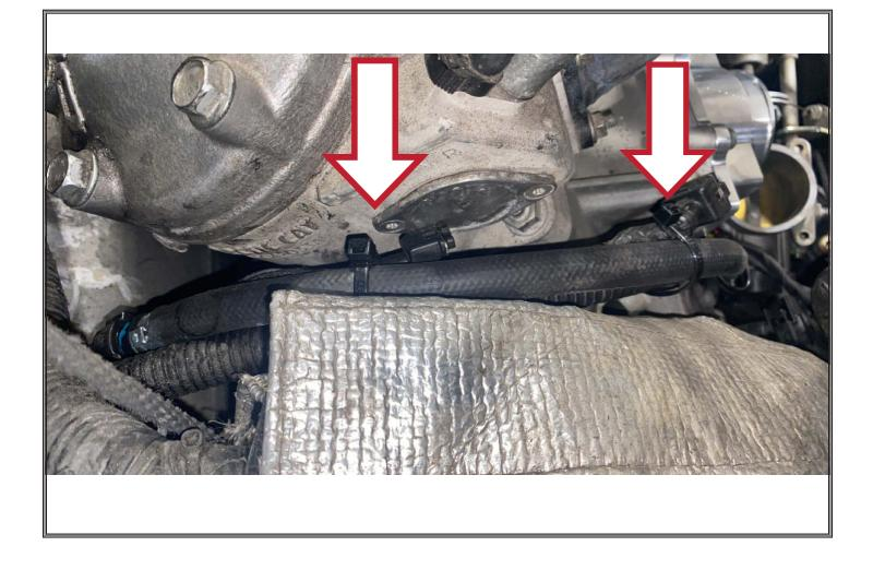
route fuel line back to OEM Fuel connector previously rotated on page 21 \*NOTE: ensure to fasten OEM injector connectors as shown to prevent interference with jack-shaft
