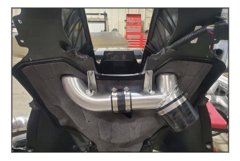
Inatall Boondocker intake plenum intt hood and secure with supplied hardware.
