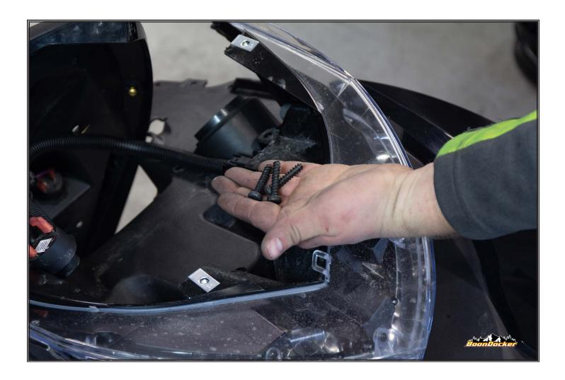
Remove 3 screws holding guage cluster/vent to hood and remove cluster.
