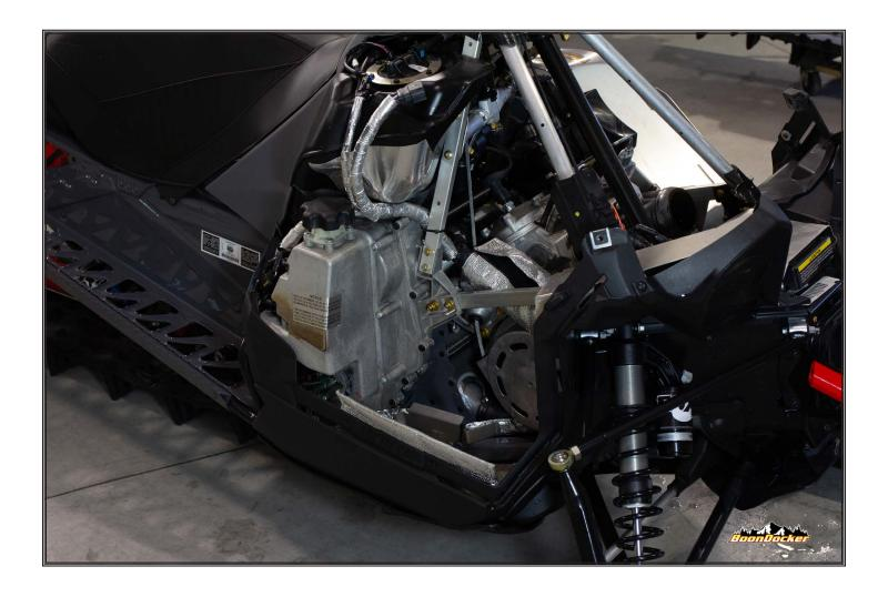
Remove tune pipe and muffler.
