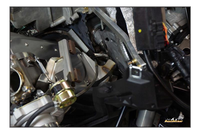
2018-2019 Models: See "2018+ Arctic Cat M8000 Sidekick Intstrucions" steps 14-21 for connecting oil lines. 2020+ Model Only: Place turbo/muffler assembly in sled. Route oil line to pump and route coolant lines to throttle bodies.
