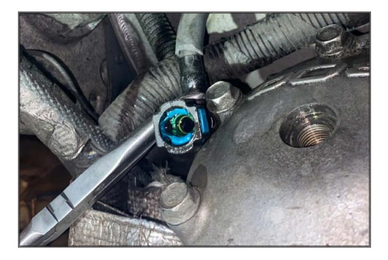
Grip OEM fuel liine at the barb and twist 90 degree fitting to point towards front of snowmobile. \*CAUTION: BE VERY CAREFUL NOT TO TWIST FUEL LINE IT WILL BREAK ONLY TWIST THE CONNECTOR\*
