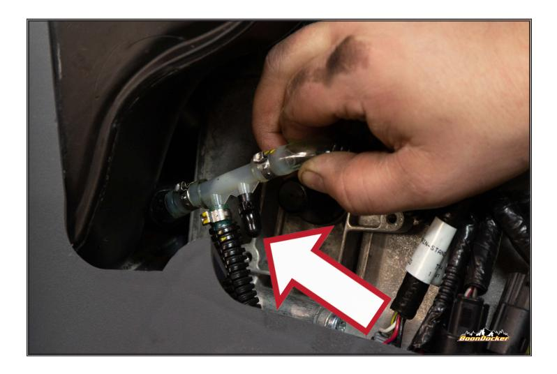
2020+ Model only. locate plastic nipple fitting. Remve line on right side and replace with supplied ruber block off. Fasten with 4" supplied zip tie.
