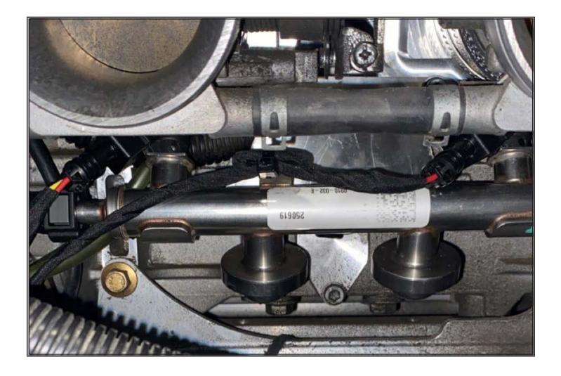
Install injector relocate harness and secure as shown. NOTE: ensure oil line clearance behind fuel rail bracket.
