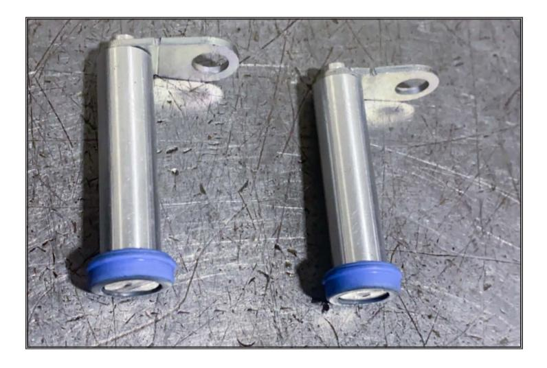
Install previously removed OEM injector rings to supplied injector plugs as shown.
