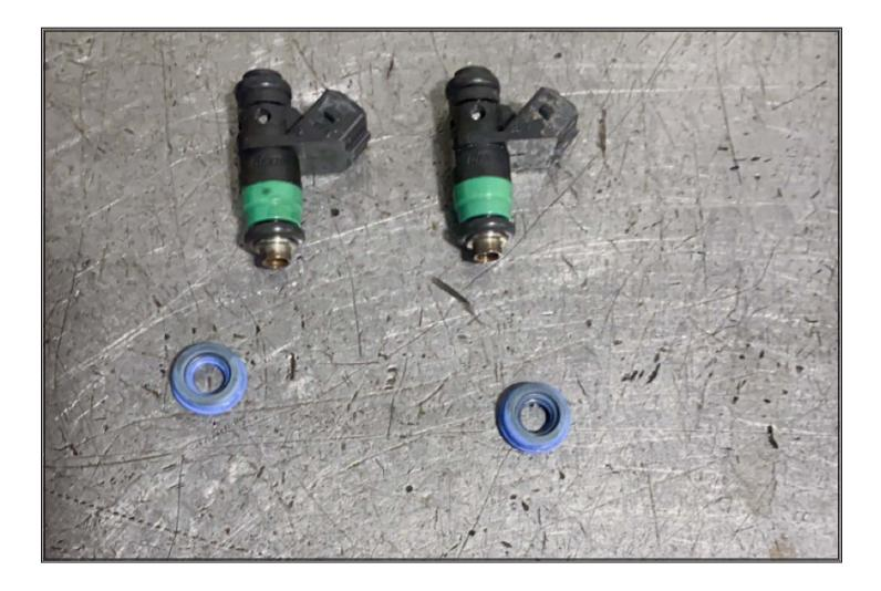
Remove OEM fuel rail and injectors from the back of the cylinder. Remove blue (or green) o-rings from OEM injectors and replace with supplied black o-rings.
