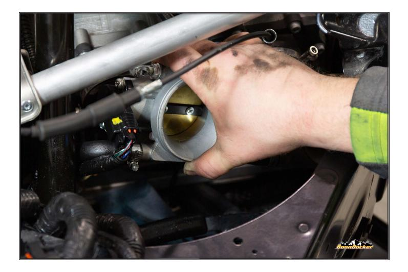
Install turbo coolant line to throttle bodies.
