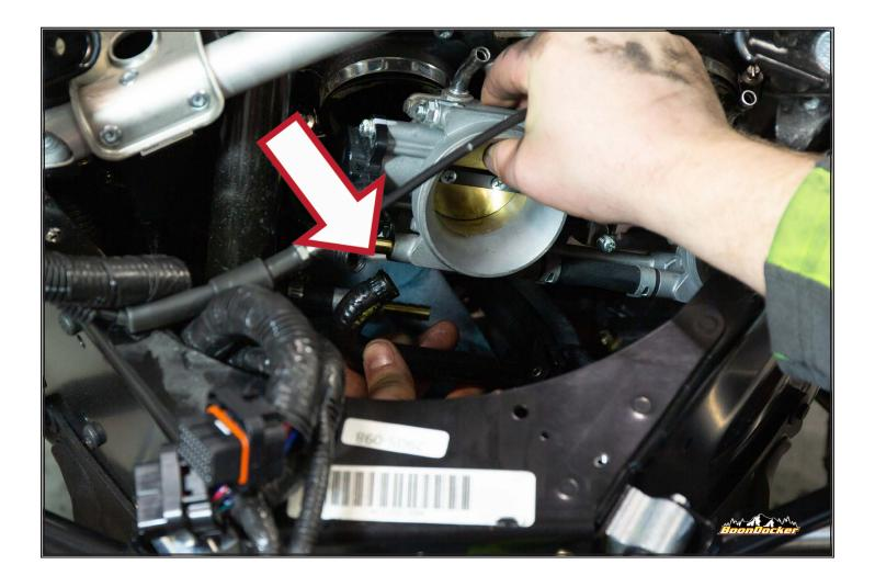
Disconnect coolant line from throttle bodies and cut 2" back, effectively removing elbow.
