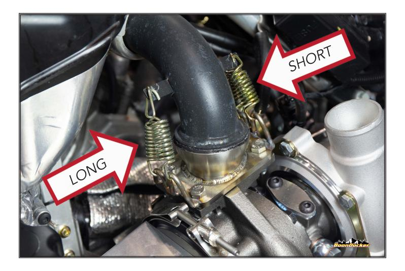
Spring tune pipe to turbo using the provided short(2) and long(2) gold springs.
