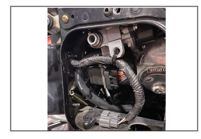
Install IAC as shown if Airbox deso not allow installation. Drill out rivet in center of bulkhead and secure with supplied bolt and nut. Install TBap as shown.
