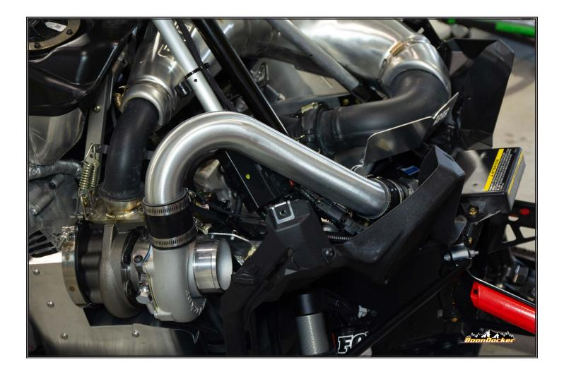
Install charge tube using suplied silicone and hose clamps.
