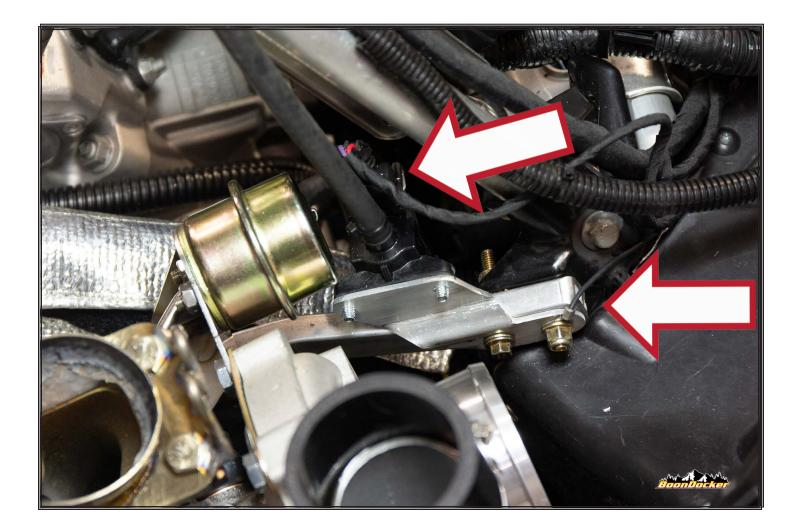
Install BoonDocker solenoid to support bar bolts located in front of turbo. Plug control box into solenoid and hook ground to front bolt as pictured.
