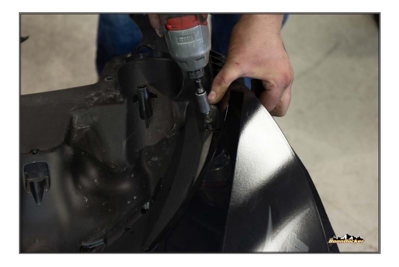
Remove 7 remaining screws holding plenum to hood and remove plenum from hood.
