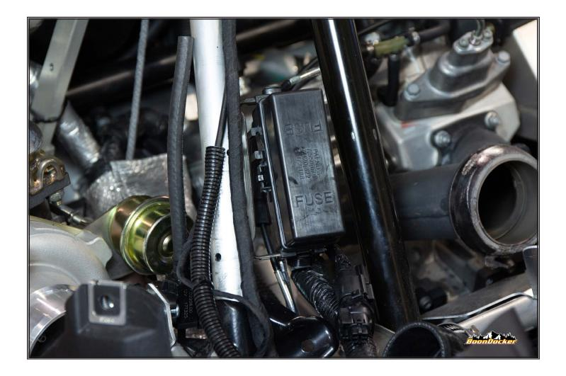
Drill rivets out of support bracket using 3/16" drill bit. Rotate approximately 90 degrees so fuse block willbe facing straight up and down. Drill new 3/16" holes and rivet back to chassis as shown.
