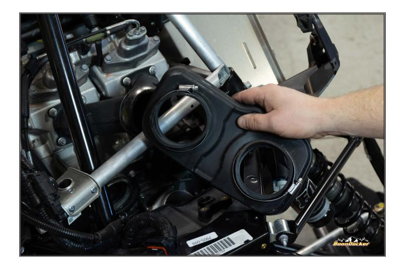
Remove airbox-throttle body grommet.
