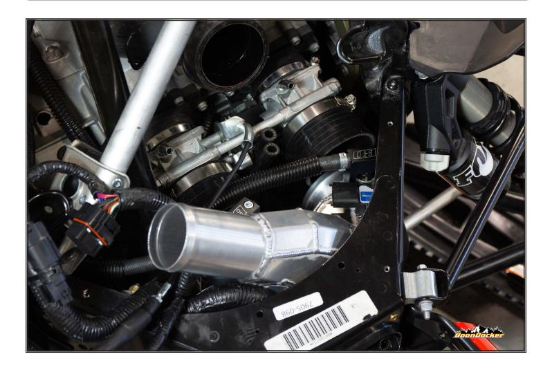
Re-install throtttle bodies and install supplied silicone to airbox.
