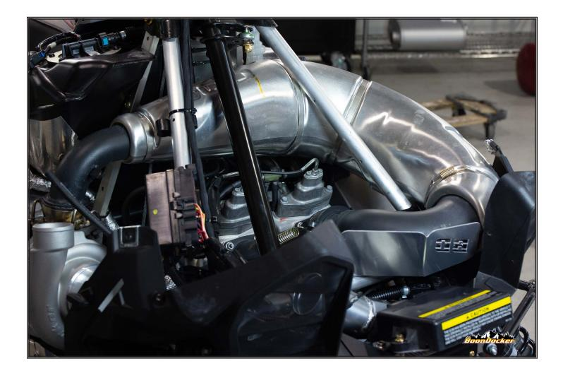
Place tune pipe back into chassis.
