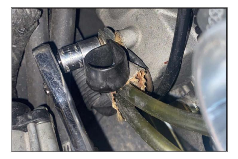
Remove both P-Clamps then install fuel rail assembly to throttle body adapters using OEM hardware in open lower center holes left open previously.
