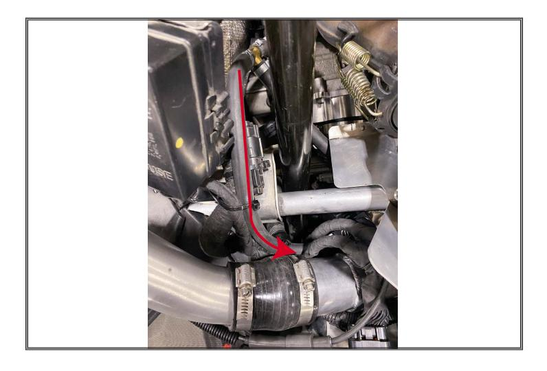
Route MAG fuel line to auxillary injector as shown. Take special care to ensure the line does not kink.
