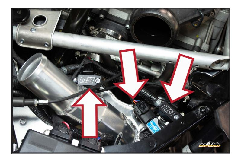
Plug in auxillary injectors and MAP sensor.
