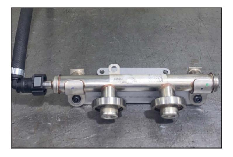
Install stock fuel rail to provided bracket as shown. NOTE: ensure to connect fuel line before installtion in sled for fitment.
