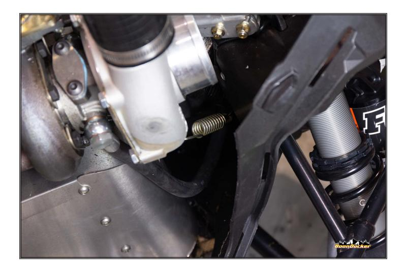
Install supplied long gold spring to front of spring tab on V-Band clamp.
