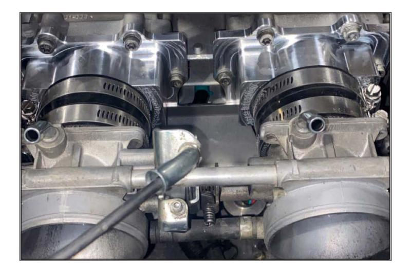
Re-install throttle bodies using supplied silicone and clamps.
