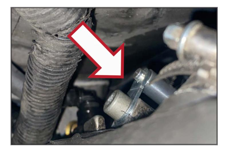
Install injector plugs in place of injectors in back of cylinder using original hardware.
