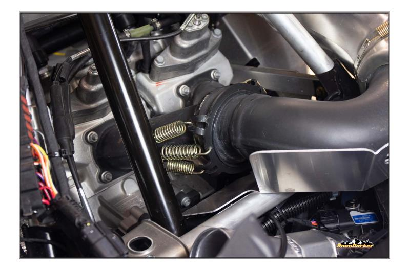
Spring tune pipe to Y pipe using 4 stock springs and two Provided fromBoonDoker kit. Drill two 1/8" holes for additional springs.
