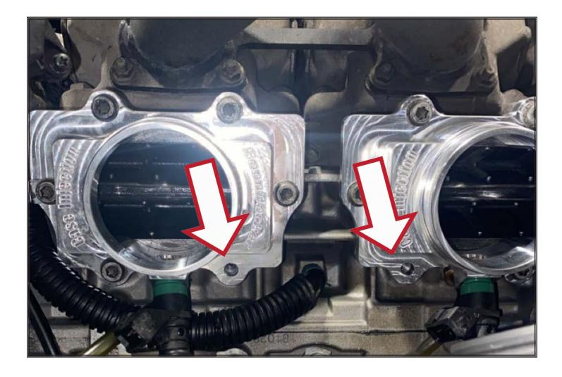
Install BoonDocker throttle body adapters leaving out lower center bolts (indicated above). Install OEM injectors as shown. \*Install reed cages in BoonDocker throttle body before installation\*
