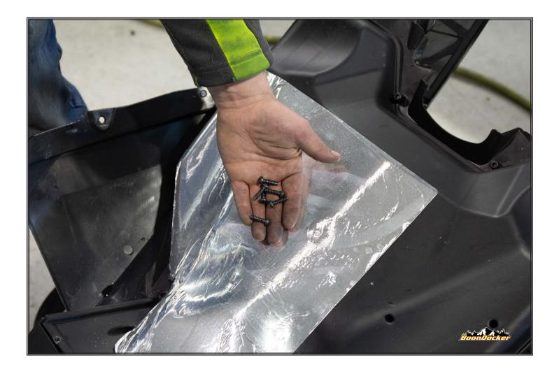
Remove 6 screws from bottom of hood.
