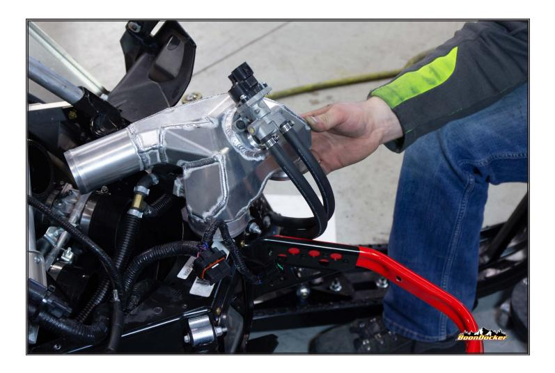
Install supplied hose to idol air control & install to airbox. NTE: if Airbox does not have place for IAC mount as shown on next page.
