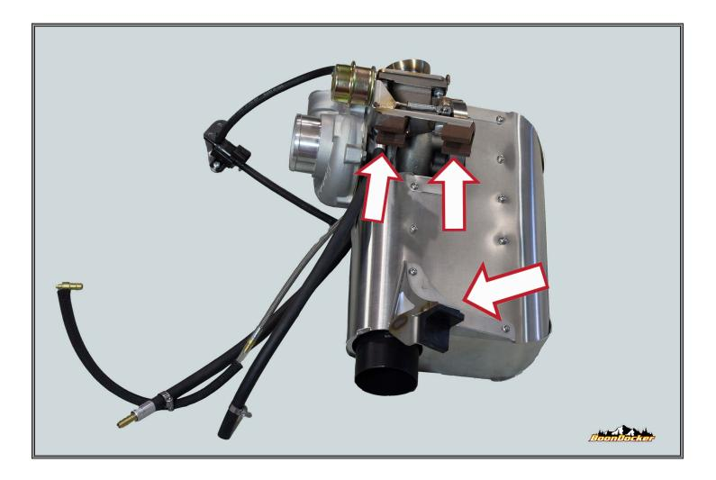
Apply stock rubber grommets to BoonDocker muffler/turbo assembly.
