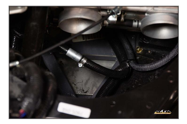
Connect barbed line from turbo to previously cut factory line as shown. Route other coolant line from turbo over to open barb on th throttle body and clamp.
