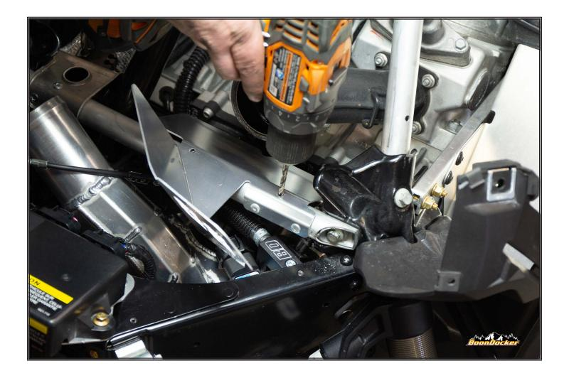
Drill two top holess with 3/16" drill bit and rivet in place.
