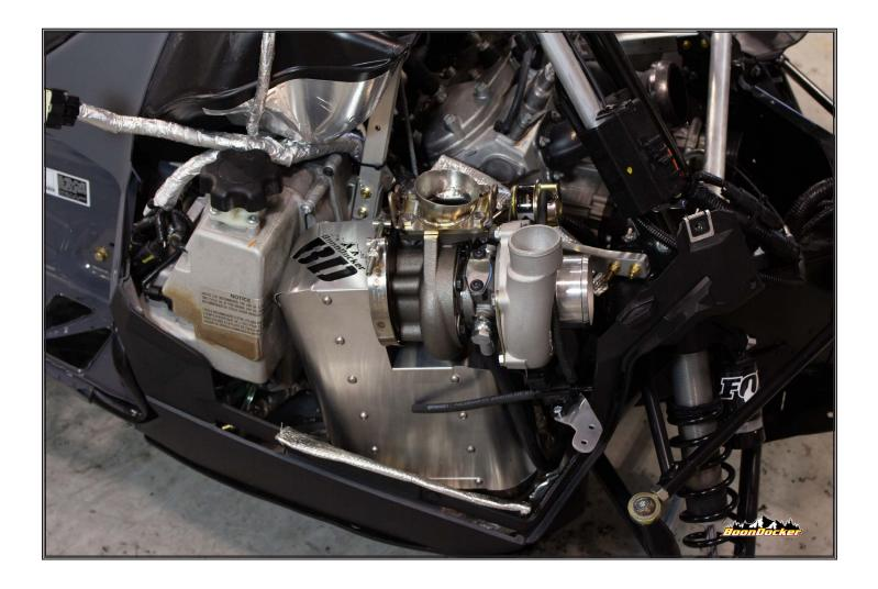
Hang turbo assembly on cross bar as shown. Ensure the turbo brackets are sitting square on top and bottom of frame before continuing.
