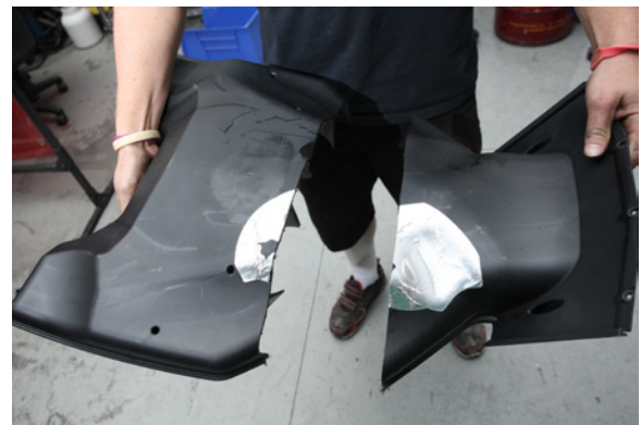
73. Cut the stock airbox in two pieces. The front section of the airbox will be discarded to leave room for the intercooler to clear.
