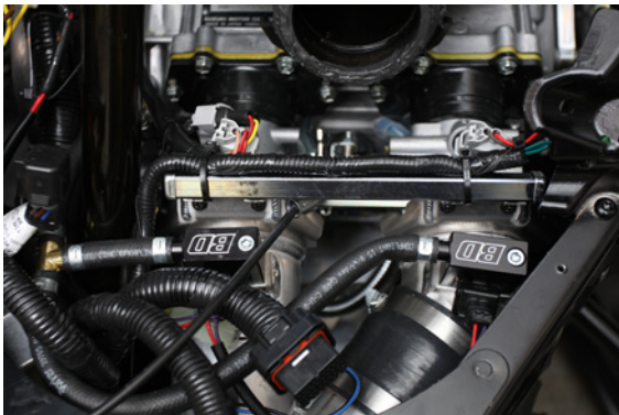
35. Plug the Control Box injector harness into auxillary injectors. Unplug the stock injector connectors and plug the matching CB injector harness connections inline with these connectors. Unplug the Throttle Position Sensor on the MAG end of the throttle-bodies and plug the matching CB injector harness connectors inline.
