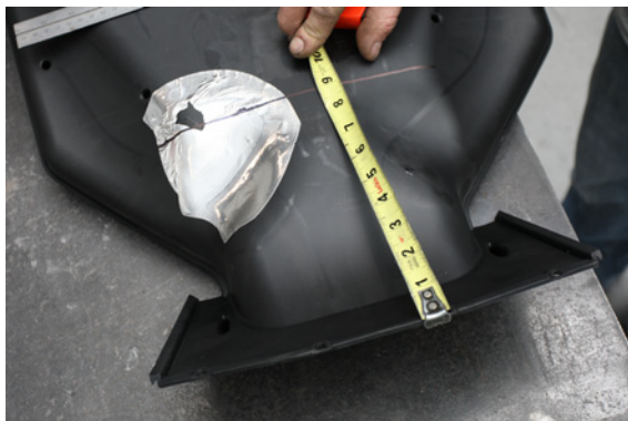
72. Measure 9" back from the front of the stock inner airbox and mark a straight line.
