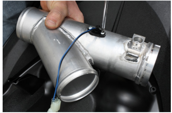
26. Seal the temp sensor with silicone and attach the temp sensor to the torque tubes using the supplied screws.
