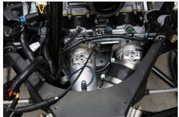
30. Move the MAG side torque tube into position and attach it to the PTO side torque tube using the 3"x3" silicone tube. Attach the torque tube to the throttle body and secure using the keeper flange.
