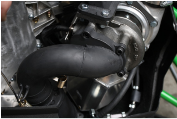
69. Using the five supplied allen head bolts secure the exhaust outlet to the turbo. Secure the exhaust outlet to the muffer using the three supplied short spring.
