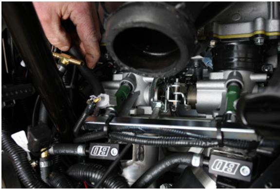
33. Locate the stock fuel line feeding the stock fuel rail. Measure approximately 1-1/2" back from the fuel rail and cut the fuel line.
