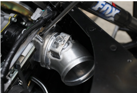
29. Install the keeper flange onto the torque tube and secure it with the stock fasteners to the fuel rail.
