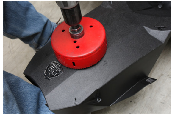
71. Measure 5-1/2" back from the front of edge of the hood and drill a 5-3/4" hole in the hood so that the intercooler fan will clear.
