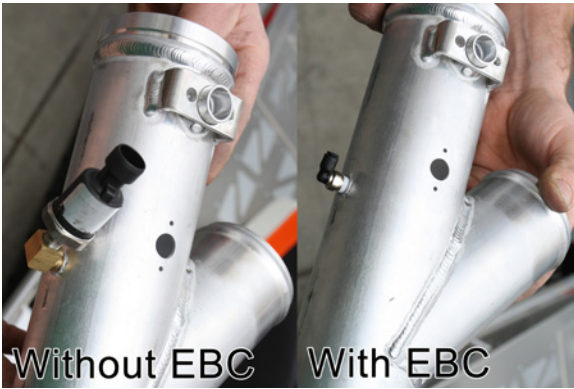
27. Install either the 90 push to connect or transducer into the torque tubes. Kits equipped with an EBC come with push to connect and without an EBC a pressure transducer.
