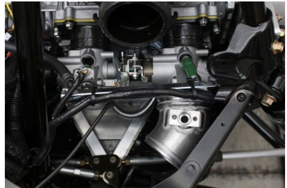
28. Install the torque tube elbow onto the PTO side throttle body.
