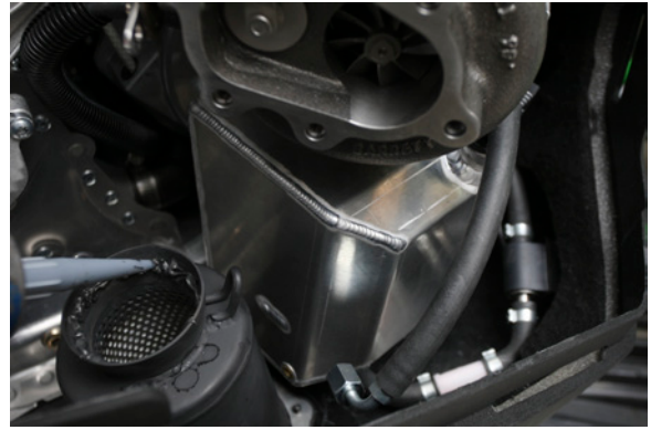
68. Install the muffer through the stock bellypan hole and add a bead of high temp silicone on the muffer ball connection.
