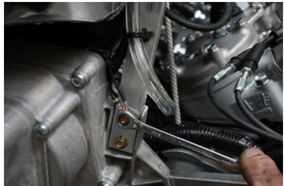
36. Unbolt the stock ground wire next to the chaincase and add the Control Box injector harness ground connector.
