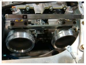
B. Insert the airbox over the machined rings. Mark and drill a 5/16" hole in the throttle body support for the airbox mount.
