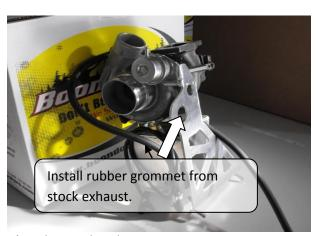
A. Mount the oil tank/ turbo assembly to the sled using the stock exhaust can mounts as shown in picture.
