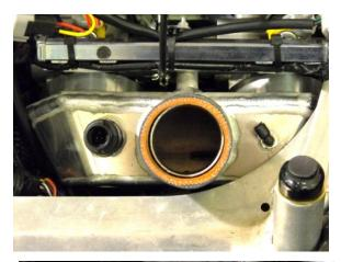
H. Push the poly line through the bulkhead fitting and connect it to the fitting on the copper cap we installed in part C.
