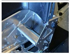
G. Cut and remove this portion of bulk head using an air saw, if you do not have an airsaw you can work this piece loose with a pair of pliers.
