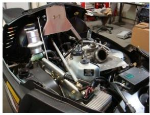
C. Remove Y pipe and heat shield. Note: If you are installing EGT's now would be the time to weld on the EGT bungs. Be sure to mount them 2 ½" from the flange.
