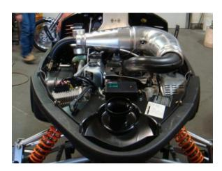
B. Remove pipe and can (remove the stock rubber mount from the exhaust can we will need this later).
