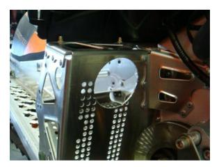
C. Using a 2 1/4" hole saw make this first cut as shown
