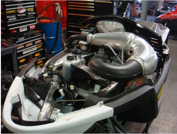
C. Remove can (remove the stock rubber mount from the exhaust can, we will need this later).
