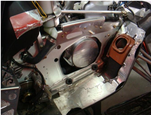
C. Remove can (remove the stock rubber mount from the exhaust can, we will need this later).
