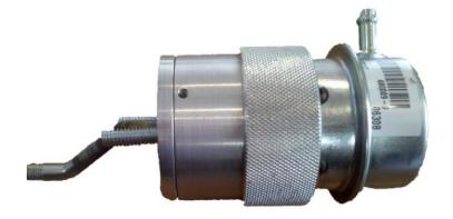
This photo represents an Adjustable Actuator that is adjusted to a maximum boost setting.
