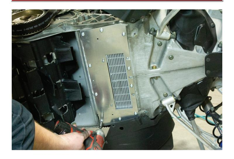
Tighten 10 Torx self threading screws using T-30 Torx bit.
