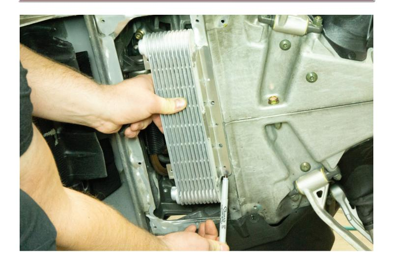
Setting cooler as shown, lining up 3/16" holes with existing holes on chassis and mark smaller holes on radiator.
