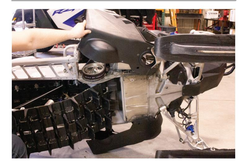
Remove plastic darts from body panels and pull belly pans away from chassis.
