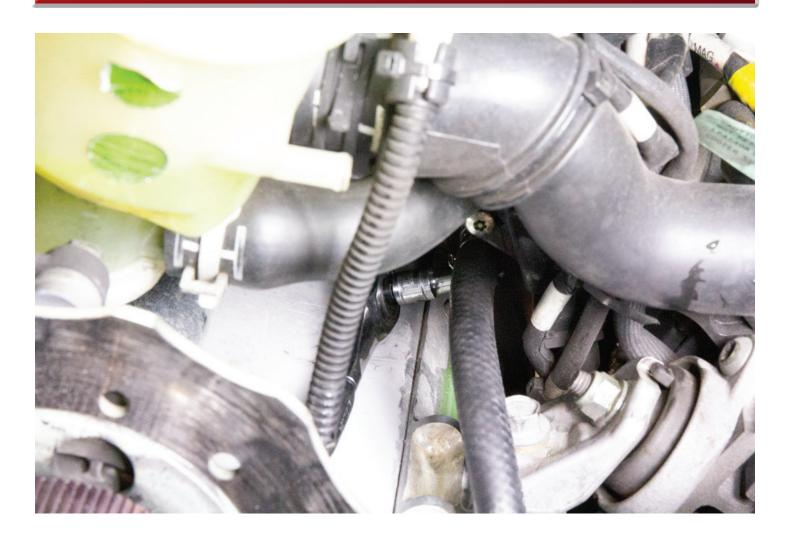
Using supplied worm clamp, install long coolant hose to throttle body.
