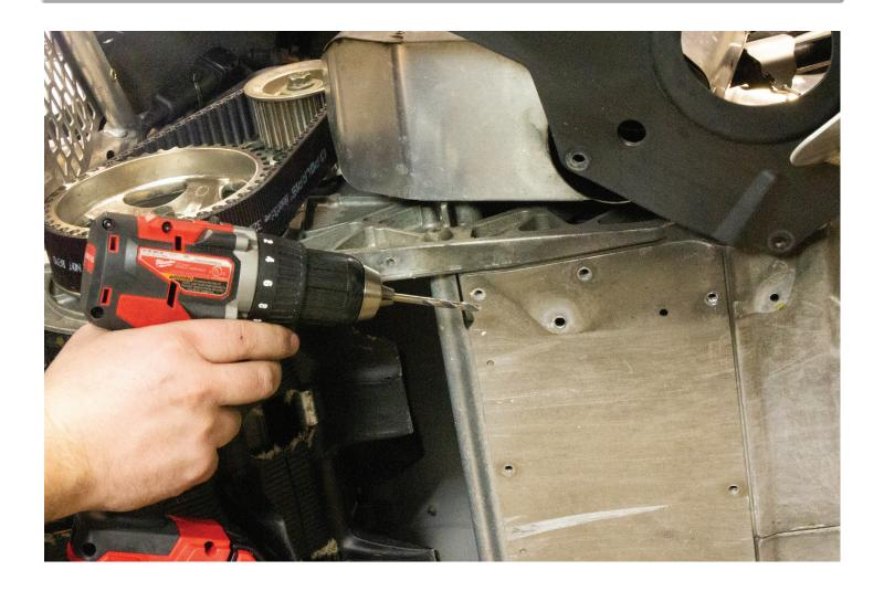
Drill out 10 rivets holding skid plate to sled.
