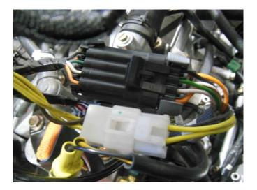
1. Locate the 8 position EFI connector (Near ECU) be sure the colors match the description below. There are 2 identical connectors near the ECU.
