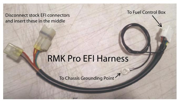
Install the EFI Harness and TPS Wire as follows. **Note:** Use Dielectric Grease in all connectors to help prevent corrosion on the terminals.
