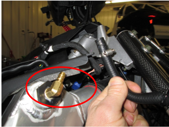
25. Swivel brass fitting upward slightly.
