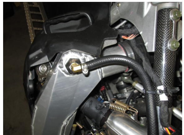
28. Attach the hose to the brass fitting and tighten. Rotate the brass fitting back parallel to outlet pipe.
