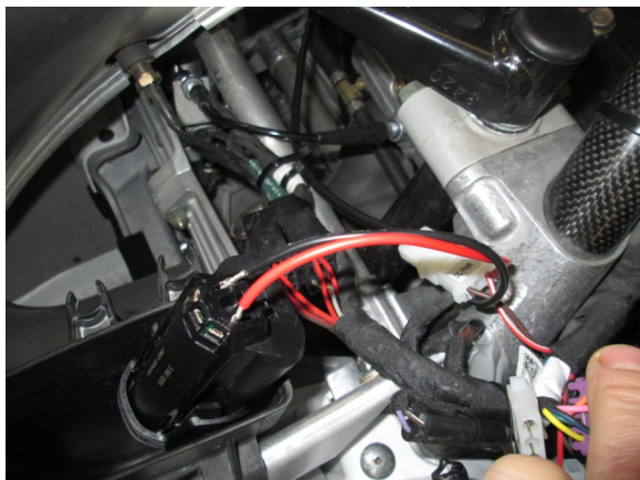
29. Use a 12 volt battery and power the pump to ensure water is pumping. You should be able to hear the pump running, let the pump run for 30 to 45 seconds.
