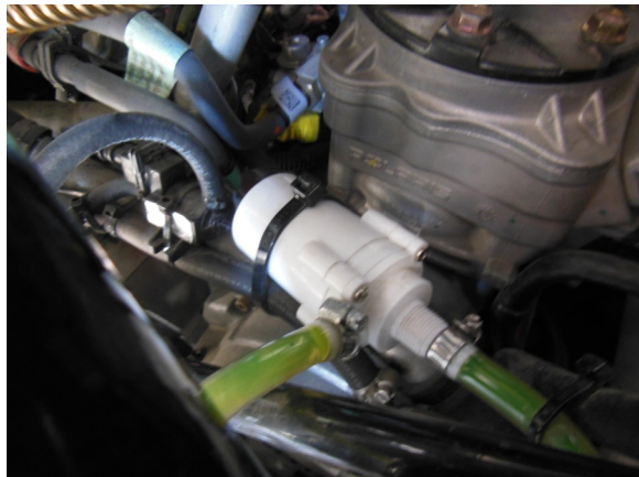
15. Secure water pump to coolant hose using large supplied zip tie as shown.
