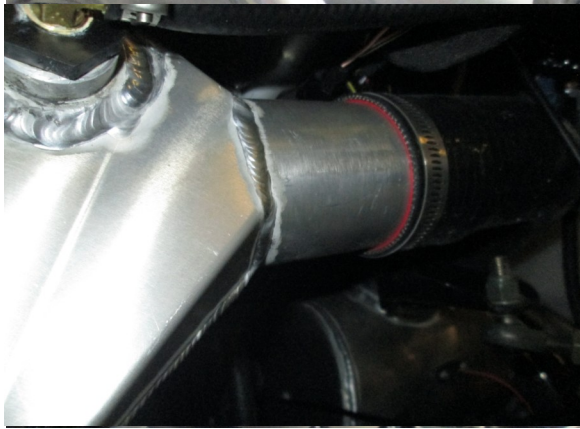
13. Slide the top of the inner-cooler into the rubber 90 coming from the air box. Make sure to slide into 90 and make sure silicone 90 is not kinked.
