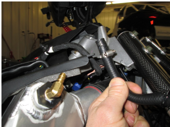
27. Hold the hose at the same level as the brass fitting. Blow into the over flow hose slowly until coolant is coming out of the hose and fitting at the same time, add coolant as needed.
