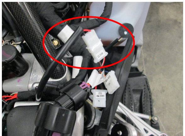
18. Make sure the electrical terminal from coolant pump is plugged into the “DC Power” terminal. Zip tie the electrical cable appropriately along the brace.
