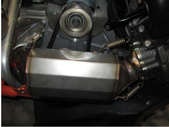
37. Install muffler using supplied springs.
