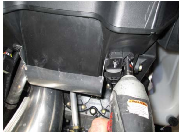
52. Insert TBAP sensor into 1/2" hole and rotate sensor to best fit. Re-use the coarse plastic screw included with the sensor and fasten sensor to air box (screw will self-tap).
