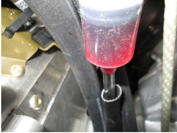
25. Using a syringe fill turbo oil feed line.
