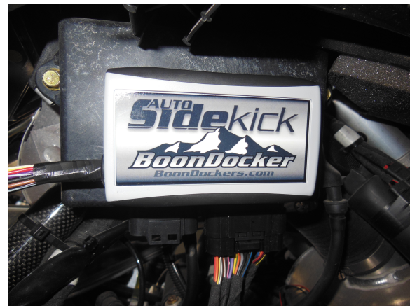
53. Plug Boondocker Sidekick box into ECU, plug stock ECU connector into control box harness. Secure Side Kick Box to the ECU using Velcro. NOTE: Zip tie harness to over structure!
