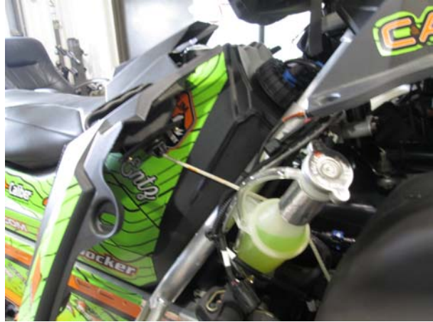
2. Remove fasteners and slide console back.
