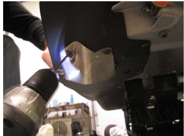
10. Remove exhaust snow deflector and muffler grommet.
