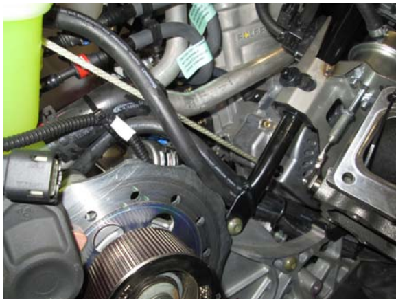
29. Route turbo coolant hoses and zip-tie as shown.
