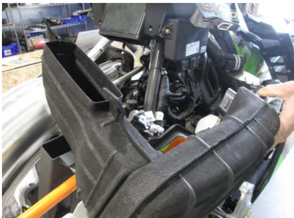
5. Remove screw, push pins, and factory ducting.
