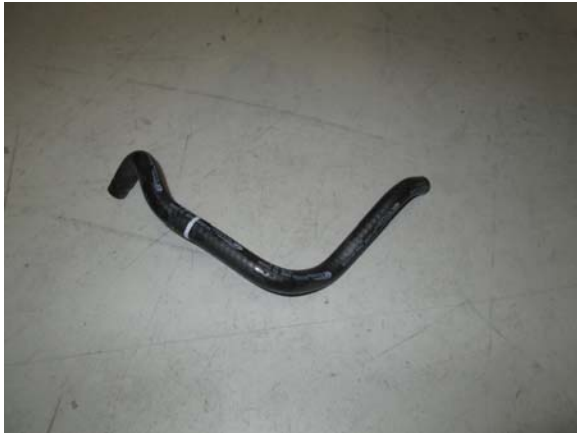
27. Remove coolant hose between coolant bottle and throttle bodies.
