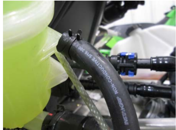
28. attach shorter turbo coolant hose to coolant bottle.
