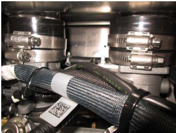
41. Set air box hose clamps loosely onto silicone.
