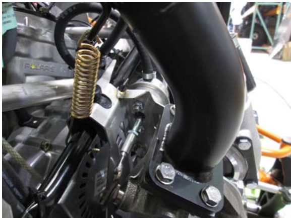
33. Use stock muffler spring to spring turbo assembly to cross bar.
