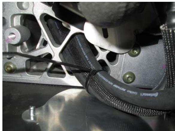
24. Route water lines and oil line through chassis and secure with a zip-tie.
