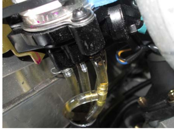
20. Cut the upper oil hose, install T and connect previously unplugged hose as pictured.
