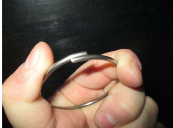
38. Bend Throttle body lock rings slightly until ends overlap.
