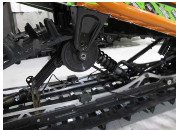
12. Hang rear of sled and remove 2 rear suspension cross shaft bolts.
