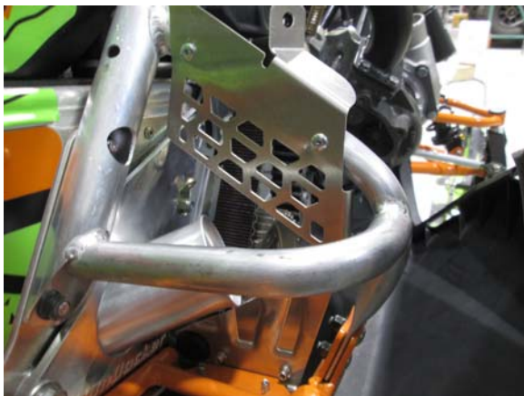
35. Reinstall kick plate using supplied rivets
