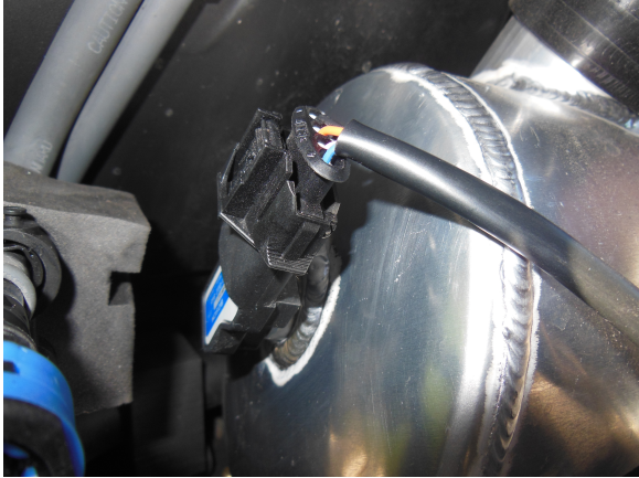
54. Connect Boondocker control box connector to pressure / temp sensor on air box.
