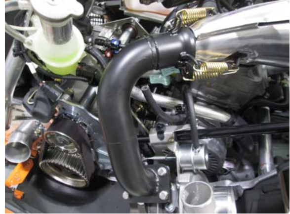
32. Install inlet with provided bolts and springs. NOTE Applying silicone to the exhaust donuts will prevent exhaust leaks.
