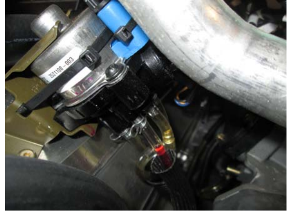
26. Re-use stock clamp from step 19 and attach turbo oil feed line to oil pump.
