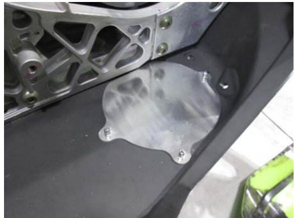
18. Rivet muffler block off plate in.
