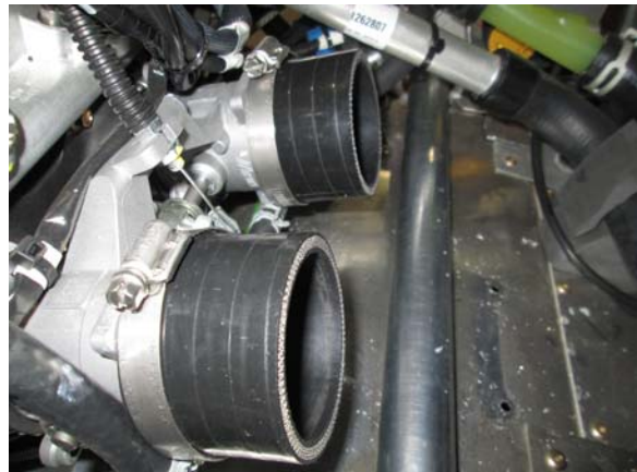
40. Install silicone onto throttle bodies and tighten hose clamps. Make sure lock rings stay in place and that the silicone and clamps are positioned all the way forward.
