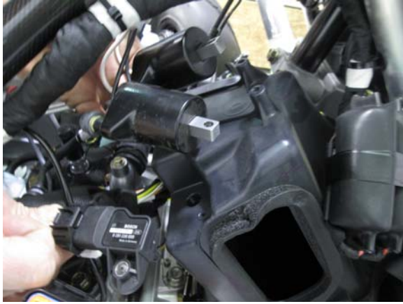
7. Un-Bolt coils, and TBAP sensor from air-box.
