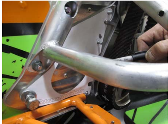
14. Cut out template and mark exhaust outlet on tunnel.
