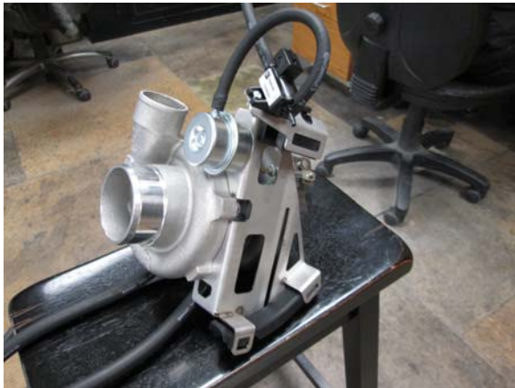
21. Install stock muffler rubber mounts on to turbo bracket. Remove and re-use screws to mount solenoid on turbo bracket as shown (electrical connection facing toward turbo).
