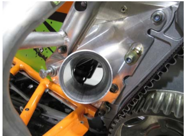
16. Install exhaust outlet tunnel support and 2 spring tabs both facing up.
