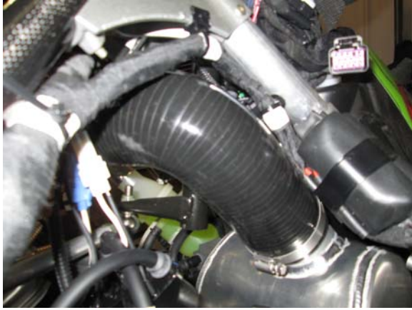
43. Install silicone 90 onto air box. Position Silicone to maintain clearance from steering.
