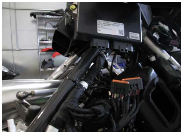
6. Unplug ECU and remove upper air-box assembly.
