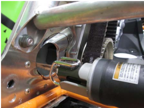
15. drill 2 1/8" hole in bottom left corner. Use a saw to finish cutting outlined hole. MAKE SURE TRACK IS CLEAR WHEN CUTTING HOLE TO PREVENT DAMAGE.
