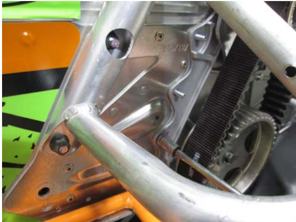
13. Remove front cross shaft bolt, and 4 belt drive case nuts.
