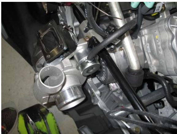
23. Mount solenoid to turbo bracket and install turbo assembly in place of stock muffler.
