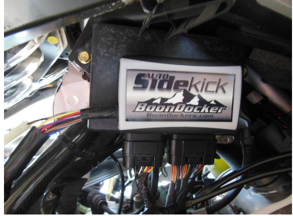
55. NOTE: Check all wire routing zip tie wiring where needed to secure and prevent rubbing or moving parts interference...
