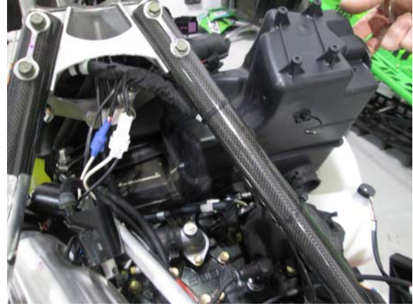
8. Remove wiring from air-box, loosen clamps, and remove air-box.
