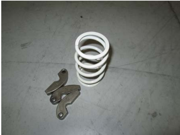
56. Replace drive clutch spring and cam arms using supplied clutch items. Supplied components are used to achieve an optimal RPM range between 8400 to 8600.
