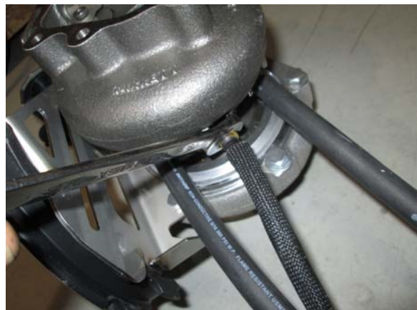
22. Connect oil feed hose to turbo.
