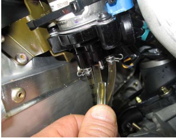
19. Unplug the stock oil line as pictured. Remove stock clamp and save for re-use in step 26 for installation of turbo oil feed line
