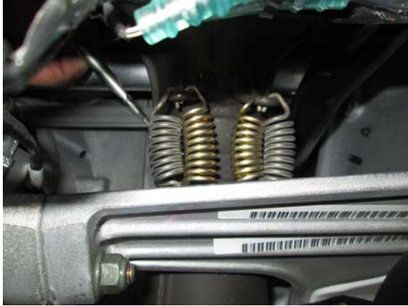
31. Using 3 of the provided short springs, Double spring tune pipe to Y pipe.
