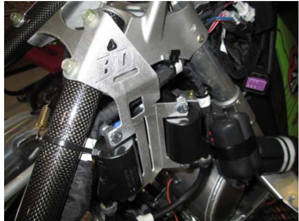
46. Install coils to coil bracket and install bracket as shown.
