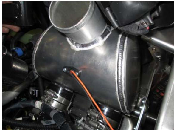
42. Install air box and tighten clamps. Make sure the top tube on the air box has enough room for silicone and clamp to slide on without rubbing the sub frame.
