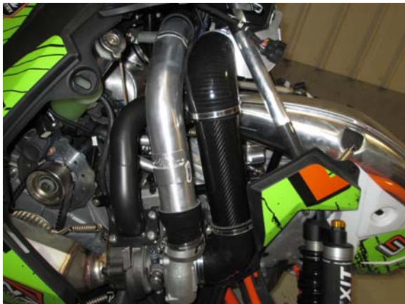
51. Install cold air box and connect plenum to tube using 90 degree silicone and tighten all clamps.
