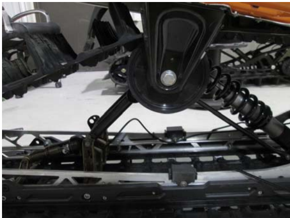
17. Reinstall rear suspension bolts.
