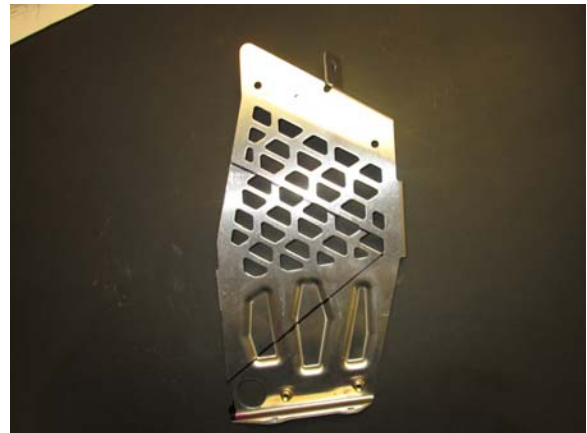
34. Measure 1" from bottom. Use a straight edge to draw a line from measure point to bottom right corner of grate and cut as shown leaving 3 grated lines above the cut mark.
