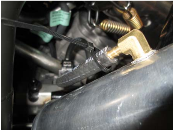
45. Connect hose coming from boost solenoid to barb on back side of the charge tube and secure with zip-tie.
