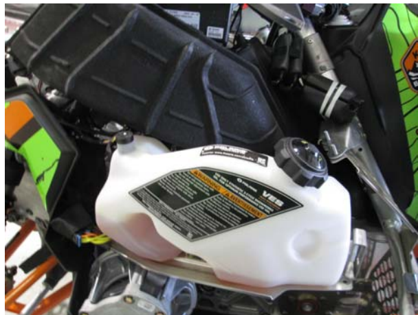
4. Remove clutch cover/ oil-tank and let rest in place as shown.
