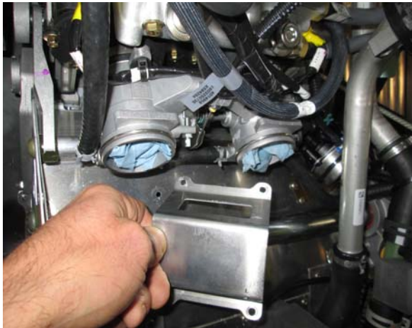
39. Snap lock rings onto throttle bodies. NOTE: {If installing SideKick X or GT Kit, Remove Air Box Support Bracket for injector clearance.
