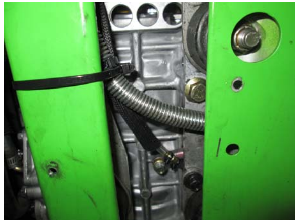
36. Routing is crucial, zip tie and secure to prevent rubbing, kinking or melting.
