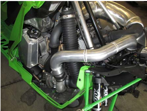
47. Install cold air intake flex hose. Ensure routing of pressure hose from charge tube and wiring from control box is secured to the bracing (see step 46).
