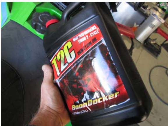
53. MUST pre-mix first tank of fuel 50:1 and verify that the sled is using oil properly to prevent damage. Discontinue pre mix after oil consumption is verified.
