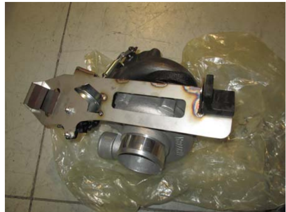
30. Remove the stock rubber mounting hardware from the stock muffler and install onto the turbo bracket.
