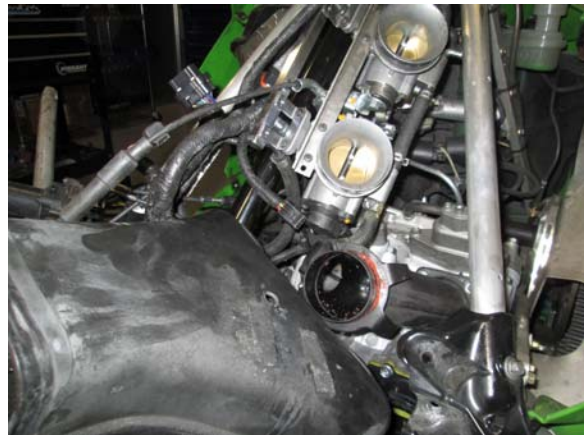
6. Move throttle bodies out of the way and remove the air box. NOTE; IF INSTALLING MTA OILLESS TURBO PROCEED TO STEP 14
