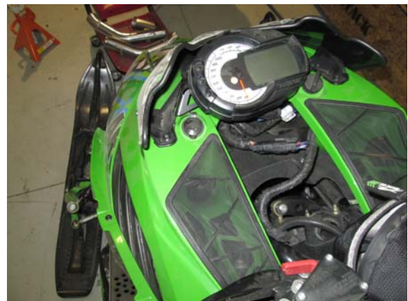
54. Set the hood in place and plug in, verify the machine starts, check that oil pump is pumping oil to the turbo and throttle bodies, run long enough to verify and check coolant level!!
