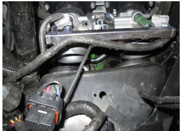
4. Loosen the clamps on the air box and slide forward to remove throttle bodies
