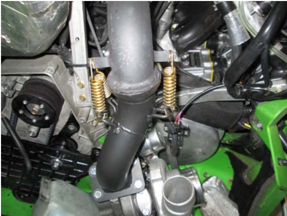
33. Install exhaust inlet onto turbo using hardware. Align and connect to turbo with exhaust pipe and install using long gold exhaust springs.
