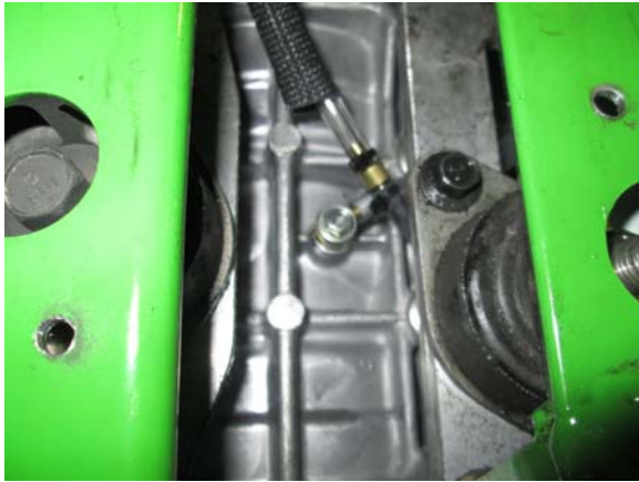
37. Install banjo fitting into crank case oil feed line and bolt to crank case (1 washer on each side of fitting).
