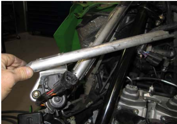
3. Remove cross brace. Unplug the servo motor and carefully move out of the way so air box can be removed
