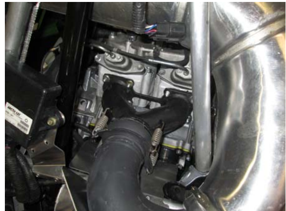
28. Apply high temp silicon to exhaust doughnuts and install the pipe using the supplied long gray high tension exhaust springs (long side of hook towards the engine, fill with silicone).
