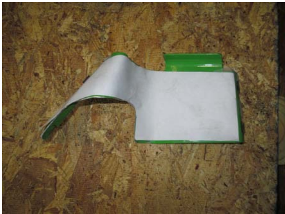
39. Using the supplied template, cut and modify the foot rest kick plate.
