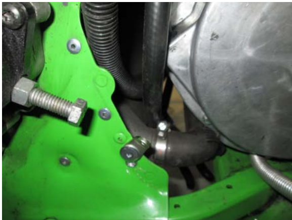
29. Drill and remove chassis rivet at this location for spring tab. Rivet spring tab to the chassis for turbo hold down.
