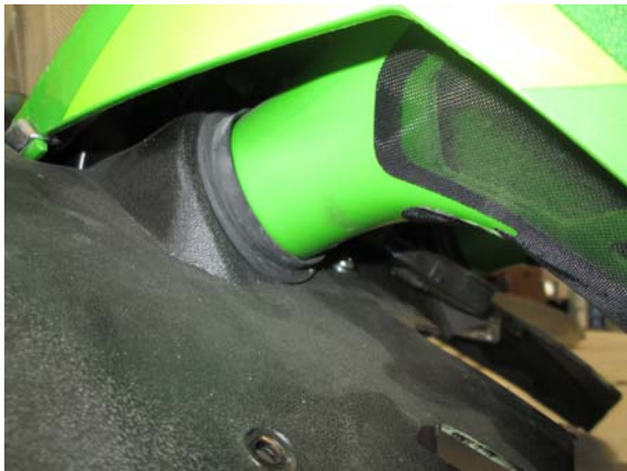
51. Re-assemble hood, be sure that the air intake rubbers are installed properly in the hood.
