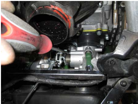
5. Unclip oil pump linkage rod, loosen clamps and slide throttle bodies out of boots. Remove coolant lines from throttle bodies, clamp or plug lines (coolant lines re-routed in Step 15).
