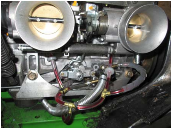
15. Install throttle body and tighten. Make sure to attach OIL LINKAGE ROD. Verify linkage operation and oil line routing, zip tie to prevent kinking and rubbing.
