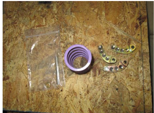
52. Load adjustable weights (if not pre-loaded) starting from heel to toe 0-2-3-3. Install clutch components (optimal RPM range 8250-8450)
