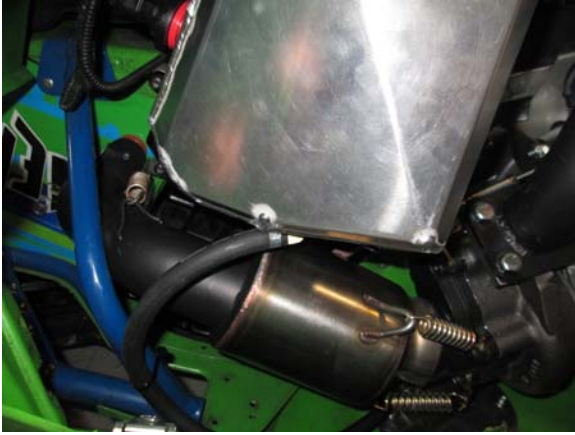
43. Zip tie oil line to the foot well upright post. Route and zip tie all wiring and hoses as far from muffler as possible.
