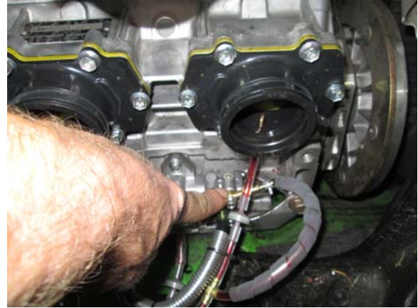
14. Rotate Banjo fitting to move hose for more clearance between throttle body and oil linkage.
