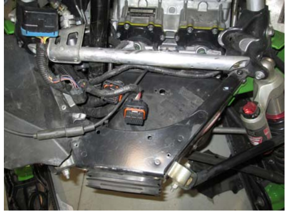
2. Remove pipe, muffler, heat shield and ECU
