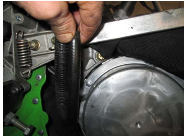
16. Route both coolant lines from throttle body (see Step 5) thru the opening between bulk head and recoil housing. (a little WD-40 will help slide hose thru clamp on bulk head)
