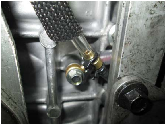
35. Connect the turbo oil feed line to the oil pump hose located on the bottom of the engine, Using a small zip tie, secure the oil pump hose to the union fitting on the end of the turbo feed line.
