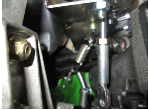
32. Tighten coolant lines and mount turbo on cross brace, spring turbo bracket into place using one long gold exhaust spring.
