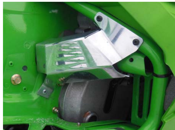
42. Install the kick plate and muffer heat shield using factory bolts, Adjust heat shield to prevent vibration and rivet into place on the tunnel.
