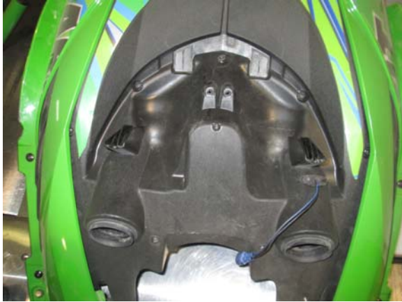
49. Remove windshield, gauge, air intake and headlight.
