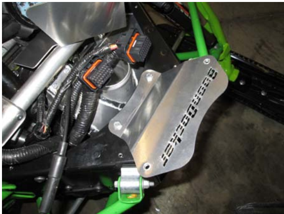
27. Install ECU mounting bracket, bolt on the ECU using the factory bolts. Re-install the two stock plastic nose wings.
