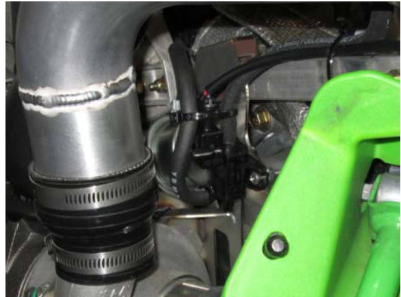
46. Install charge tube, plug in boost control solenoid, connect boost hose from charge tube, zip tie hoses and wiring to the solenoid and onto brace to keep away from heat and prevent rubbing.
