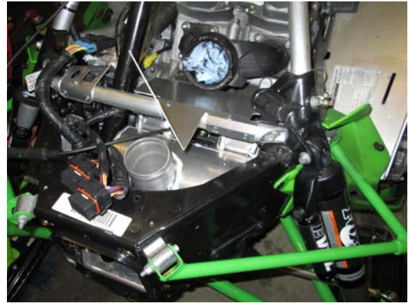
26. Install injector/exhaust heat shield, using the two predrilled holes on cross brace. Drill remaining holes and rivet in place.
