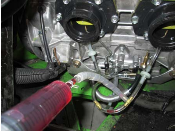
13. Before installation of last oil line to oil pump, use a syringe and fill lines with oil.
