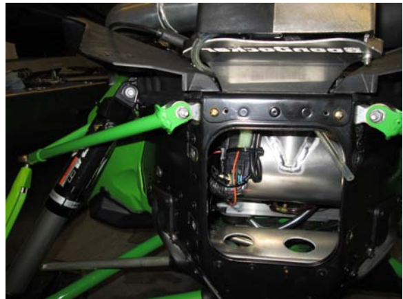
48. Routing is crucial, keep control box wiring, boost lines and boost hoses away from heat. Only place gradual bends in boost line to prevent kinking and don't over-tighten zip ties.
