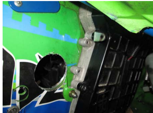
40. Remove stock spring tab from front side of chain case and place onto chain case cover using factory bolt where shown.
