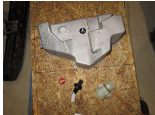
18. Drain oil into a clean container and remove the stock oil tank. Remove oil level sensor and rubber insert as well as the oil fill neck.
