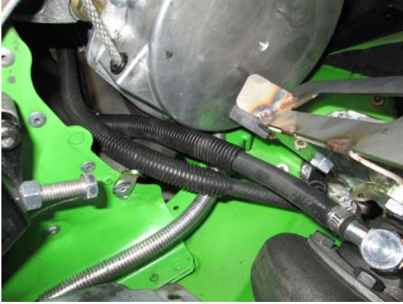
31. Hold turbo in place, route short coolant line to inside fitting on turbo, route long hose to outer fitting and cut to length. Install protective sleeve leftover from long line onto short line.
