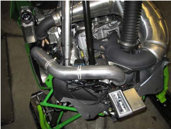
45. Install the Boondocker control box. Place supplied heat tape on ECU as shown. Connect and secure temp sensor, boost line, ECU and ground wires.
