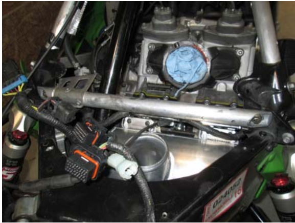
25. Install cross brace and plug in the servo motor.
