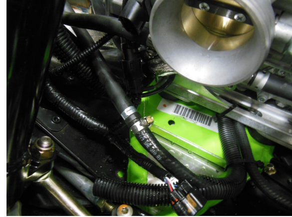
42. Connect previously cut hose to open barb from previous step. Secure with hose clamp.
