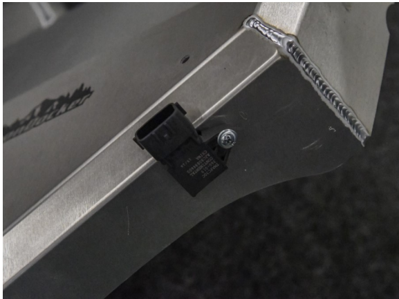
93. Install factory TBAP sensor onto BD air intake plenum with supplied self-tapping screws
