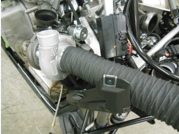
55. Temporarily install cold air intake hose to turbo to prevent debris from entering turbo.
