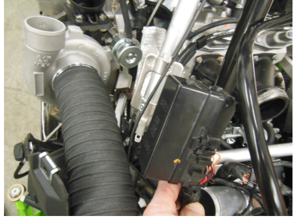
54. Fuse box needs to be relocated by rotating. Detach fuse box from mounting bracket.
