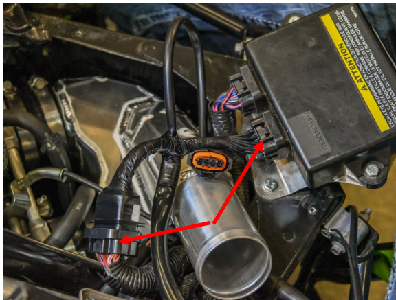
65. Route BD wiring harness as shown. Plug in BoonDocker harness to factory connector and ECU module.
