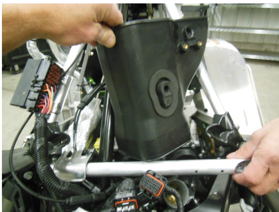
35. Remove and discard remaining airbox assembly.
