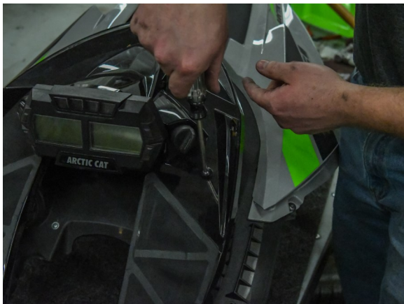
95. Reassemble gauge console using factory hardware.
