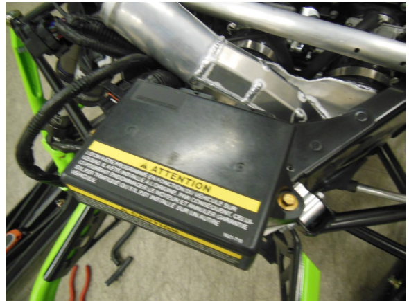
52. Install ECU onto relocation bracket using factory bolts
