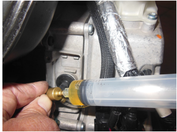
20. Using a syringe, pre-fill the oil feed lines using 2-stroke oil. Note: this line may gravity drain and may not remain full.
