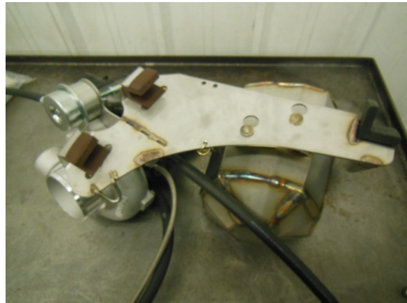
10. Install rubber mounting dampeners on turbo/muffler bracket as shown
