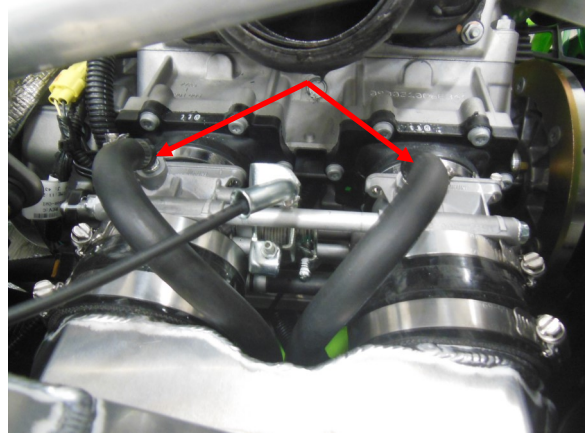
50. Install IAC lines to throttle bodies, as shown. Secure with supplied hose clamps.
