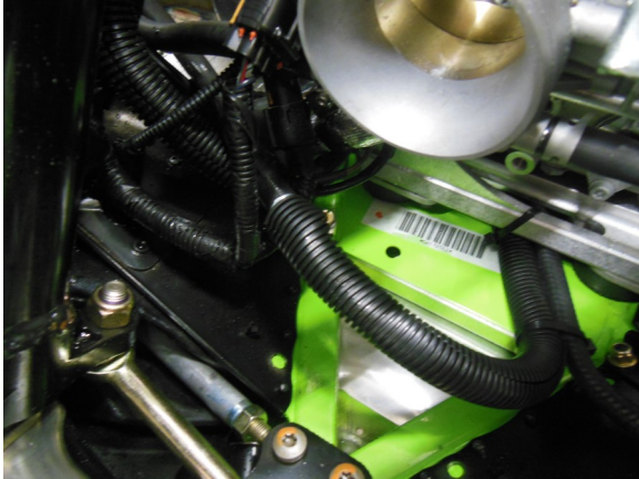
43. Slide convoluted tubing back into place to protect coolant line.
