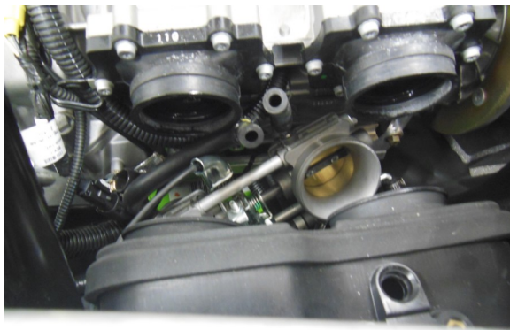
33. Loosen hose clamps securing throttle bodies to engine block, and slide forward and lay throttle bodies below airbox
