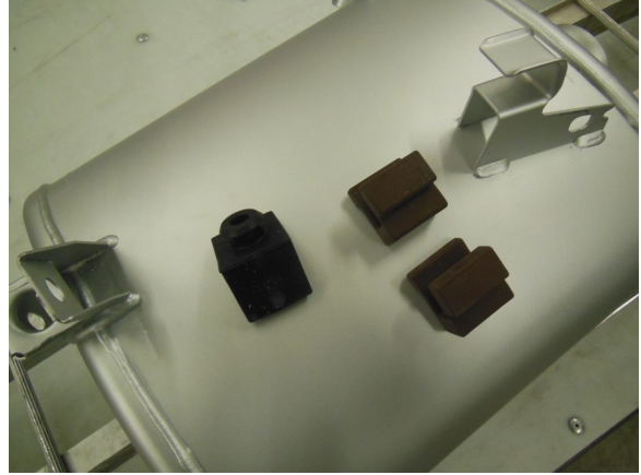
8. Remove and save the (3) rubber mounting dampeners for future use.
