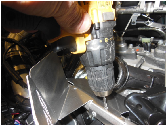
77. Drill out holes on top of heat shield and install rivets to secure heat shield.
