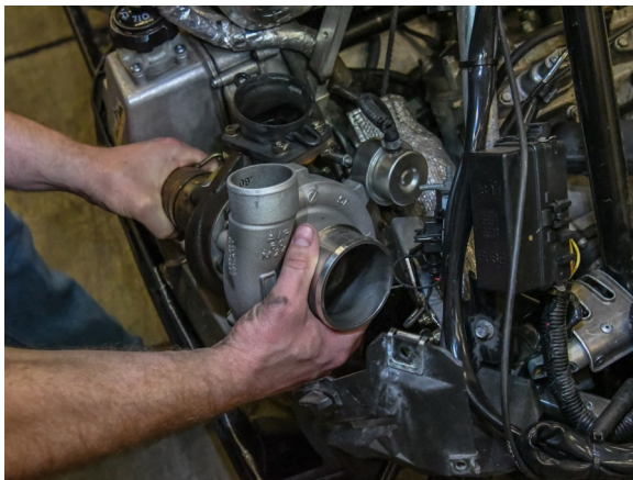
11. Slide turbo/muffler assembly into chassis. Align on cross-member
