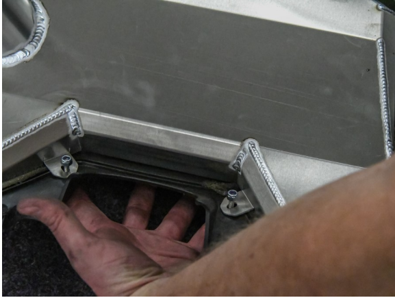
91. Attach nuts to short bolts and tighten.
