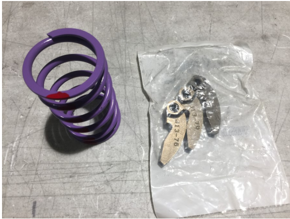
102. Install supplied weights and springs per Arctic Cat instructions.
