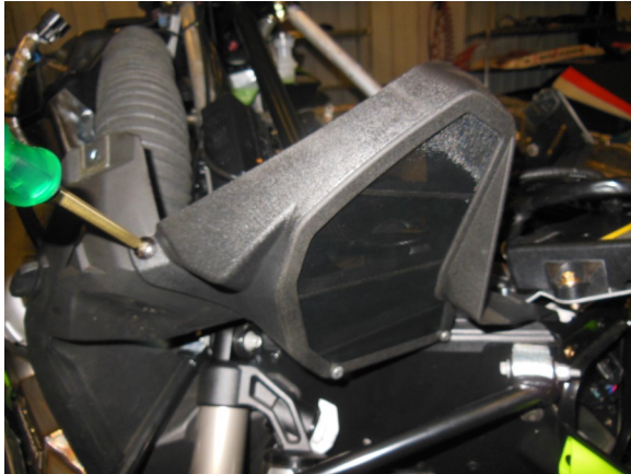
75. Reinstall factory vent shroud
