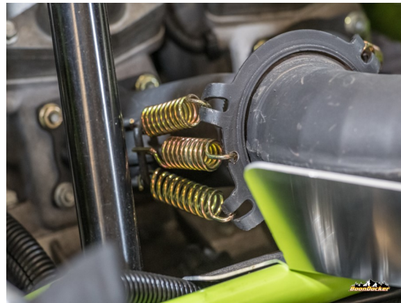
81. Install SUPPLIED (short) springs as shown, replacing 4 stock springs at each corner and adding 2 springs in the middle (6 springs total).
