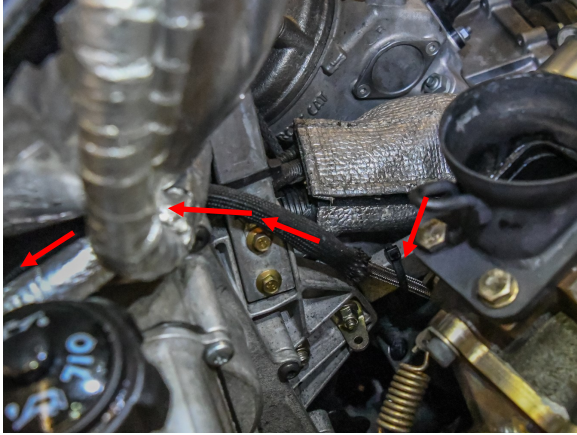
13. Route oil line as shown. Secure to cross-member with zip-tie
