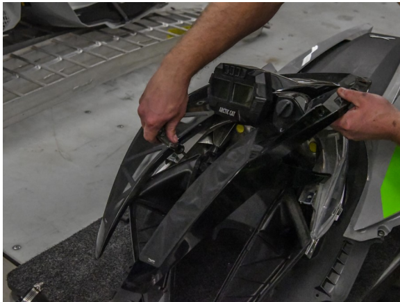
87. Remove venting for further hood disassembly
