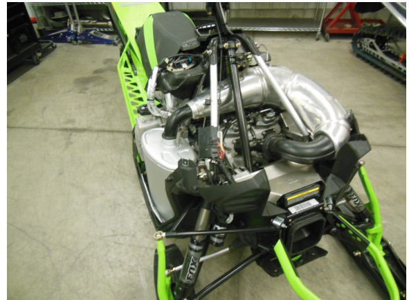
4. Release clips, unplug gauge and remove hood.
