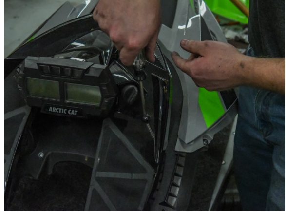
86. Disassemble gauge cluster
