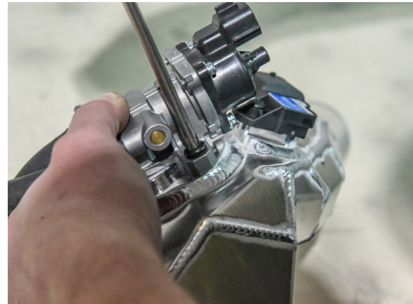
46. Install the IAC module, previously removed from airbox. SEAT the O-ring first, and hold in-place while then attaching with supplied screws. Tighten bolts to secure IAC.
