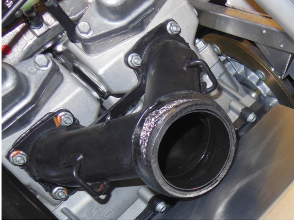
79. VERY IMPORTANT: Inspect graph-oil donut for damage. Replace as needed. Note: The above donut shows damage (wires showing) and should be replaced.
