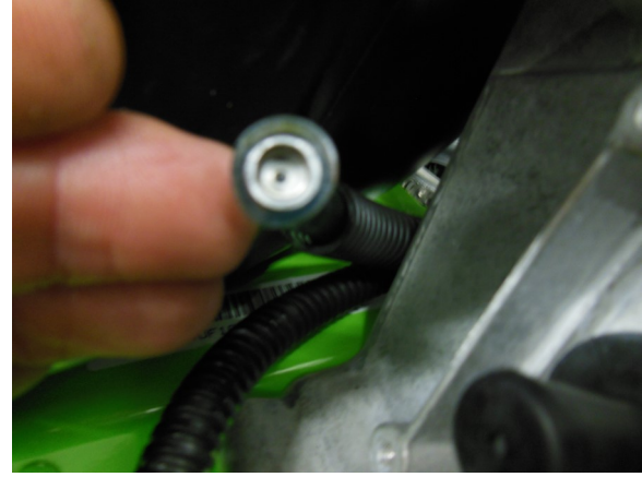
18. Install supplied restrictor plug into the longer oil line which routes to the engine.
