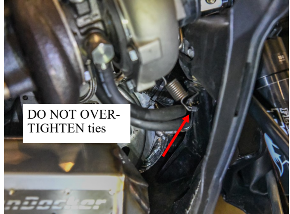
44. Secure coolant lines as shown. Zip tie to spring mounting tab. Verify routing to prevent heat penetration and friction chafing. DO NOT overtighten zip-tie.
