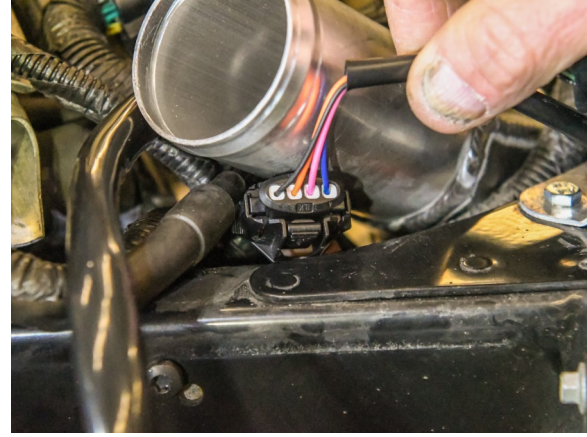
66. Route TBAP harness under air-box, down to nose-cone area.
