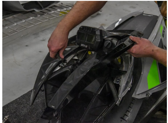
94. Re-assemble vents using factory hardware.
