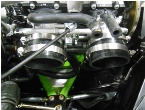
47. Install supplied intake boots to throttle bodies. Install hose clamps as shown. Secure to throttle bodies and tighten clamps.
