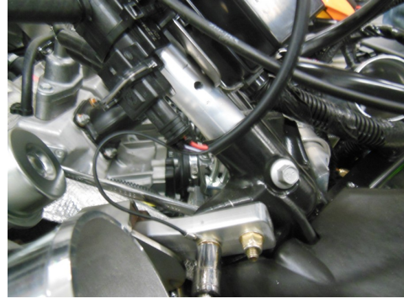
60. Remove cold-air intake hose. Attach BD wiring harness to boost solenoid.
