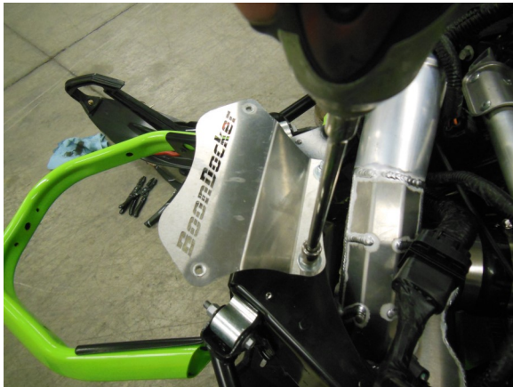
51. Install ECU relocation bracket as shown, using supplied hardware.
