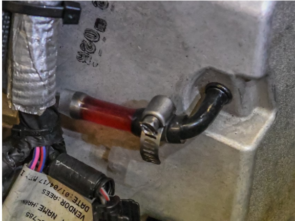
15. Install SUPPLIED block-off tubing and secure with clamp.
