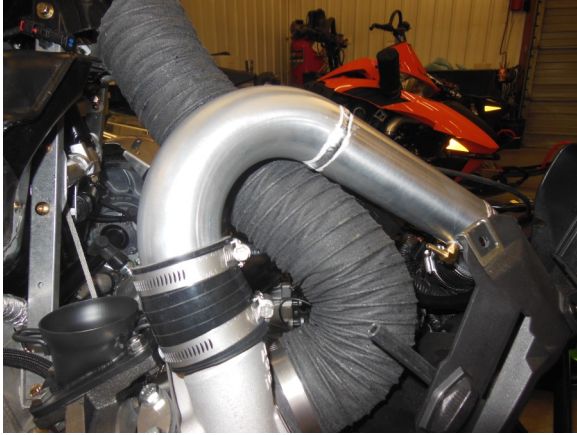
73. Route intake hose as shown. Install charge tube to turbo. Note hose clamp orientation. Tighten hose clamps. Note: boost hose may come pre-attached to fitting/charge tube.
