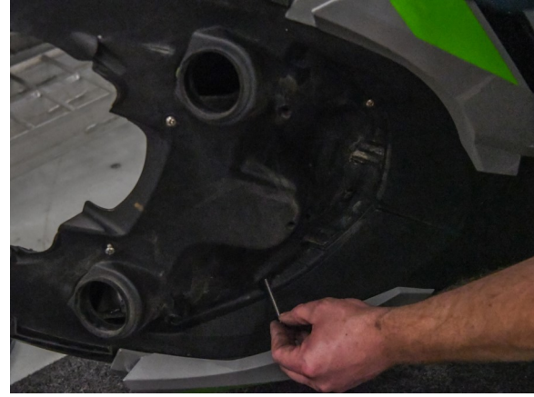
90. Use supplied hardware to attach BD cold air intake plenum to hood. Line up 4 holes in Plenum with existing holes in the hood.
