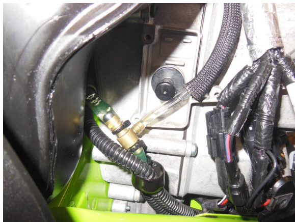
21. Connect remaining open barb on "T" to oil pump feed line. Secure with zip ties as shown.
