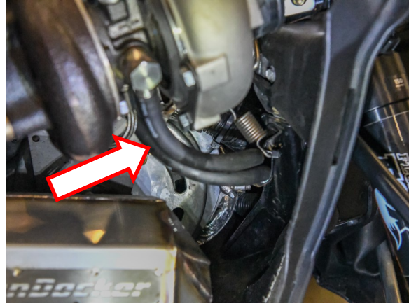
12. Route coolant lines around the front of the motor as shown. Install hold down spring as shown.
