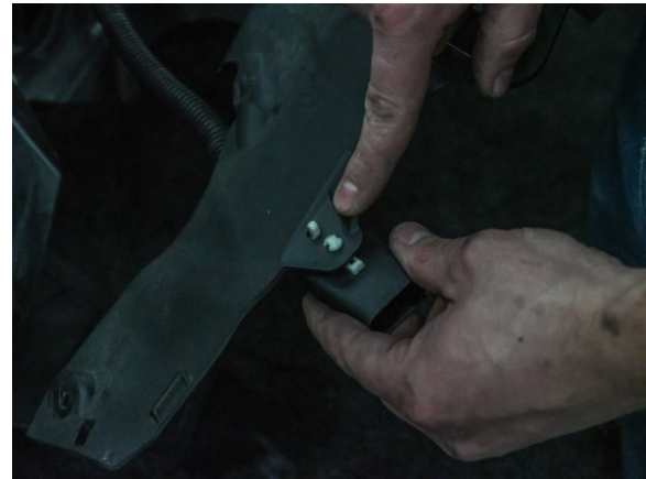
88. Disconnect wire harness from hood assembly
