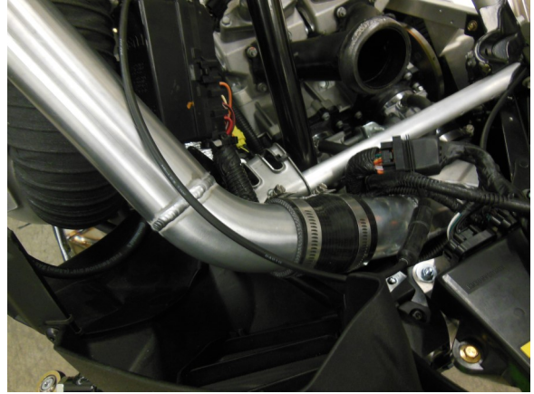
72. Install silicon coupler between air box and charge tube as shown. Take note of hose clamp orientation. Tighten clamps to secure.
