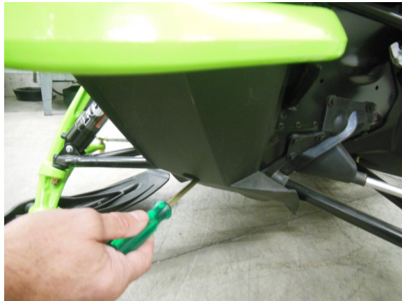
3. Using a Torx driver, remove the nose-cone hardware, and remove the nose-cone assembly.
