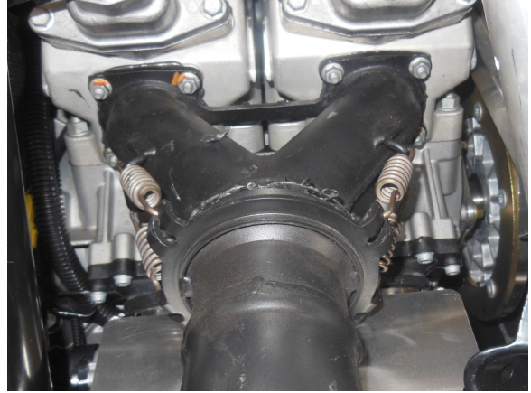
80. Drill 1/8" hole centered in pipe flange before installing pipe onto y-pipe (see step 81 for hole location). Use silicon on the inner rim of the pipe to create a good seal to Y-pipe.
