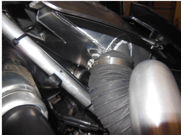
99. Reinstall hood on chassis, install BD intake hose to BD intake planum. Note hose clamp position.
