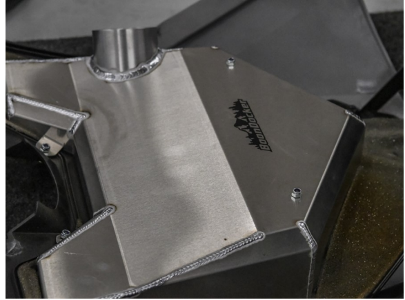
92. Install and tighten supplied hardware to secure BD intake plenum to hood.
