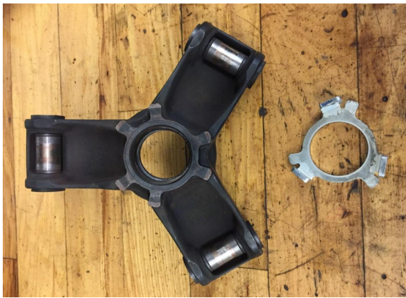
104. NOTE: some riders prefer a higher engagement. You can remove the above shim and install J13-74 gram weights to adjust your engagement.
