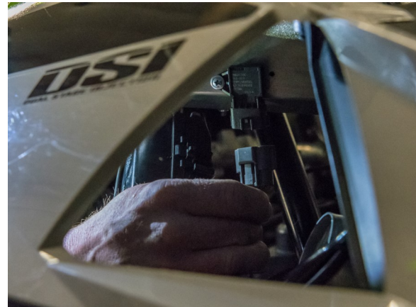
100. Install TBAP harness to TBAP sensor. Note: Some pieces have been removed to take this photo, not necessary for the installation of this harness.
