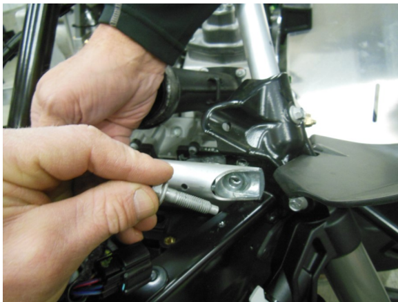
29. Unbolt cross-member and rotate counter-clockwise for additional working space.
