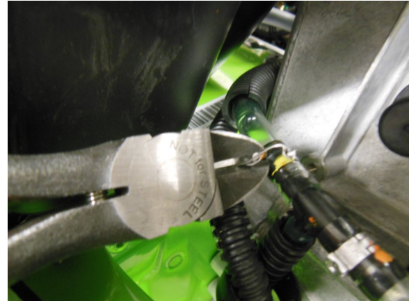
16. Cut Oetiker clamps from factory barb as shown.
