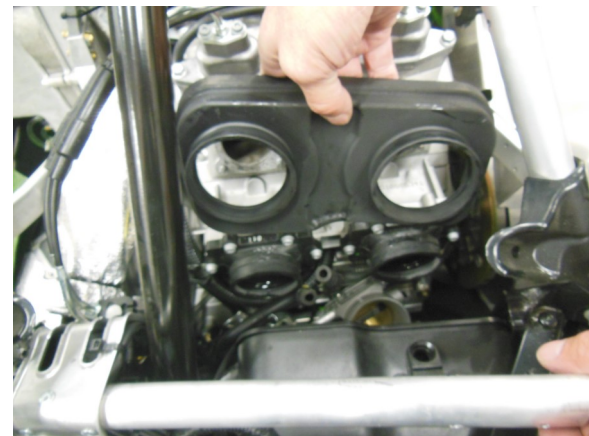
34. Remove airbox cover from airbox assembly.
