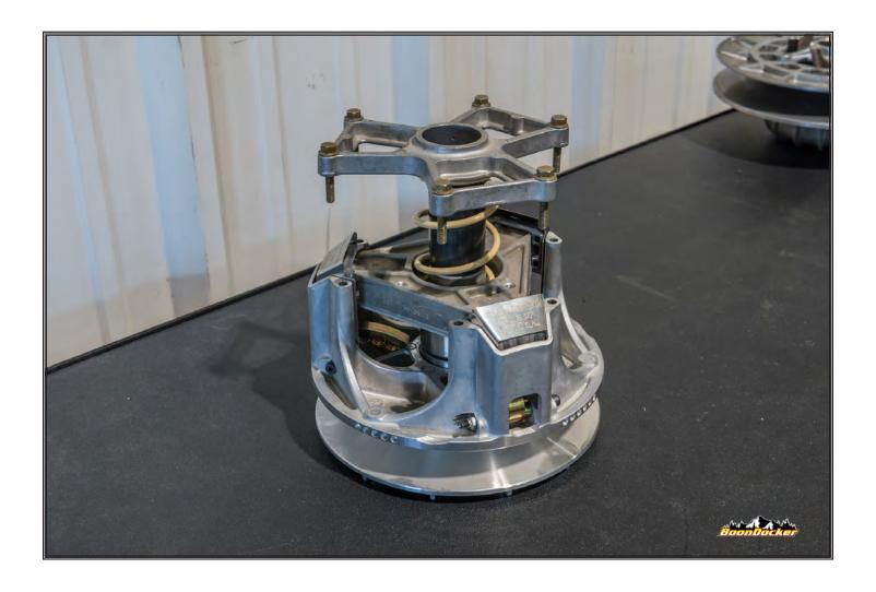
Reinstall cover to primary clutch, using supplied Tan spring. Tighten all fasteners to factory spec.
