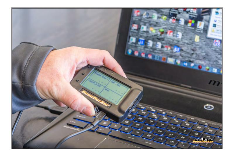
Using the supplied Micro-USB cable, plug the PVCX into your computer.
