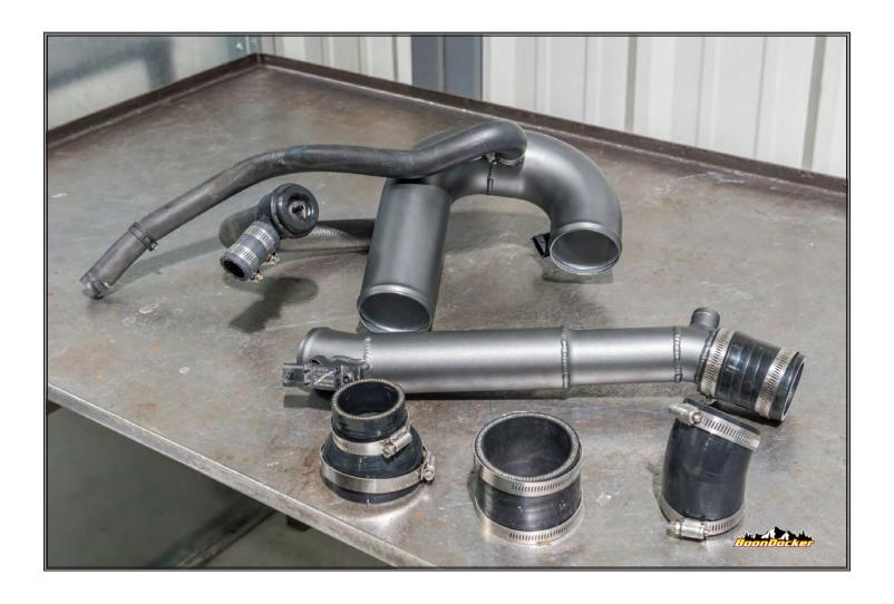
Loosely install hose clamps on silicone fittings. Install silicone fittings on blow-off valve, cold air intake, and charge tube as shown.
