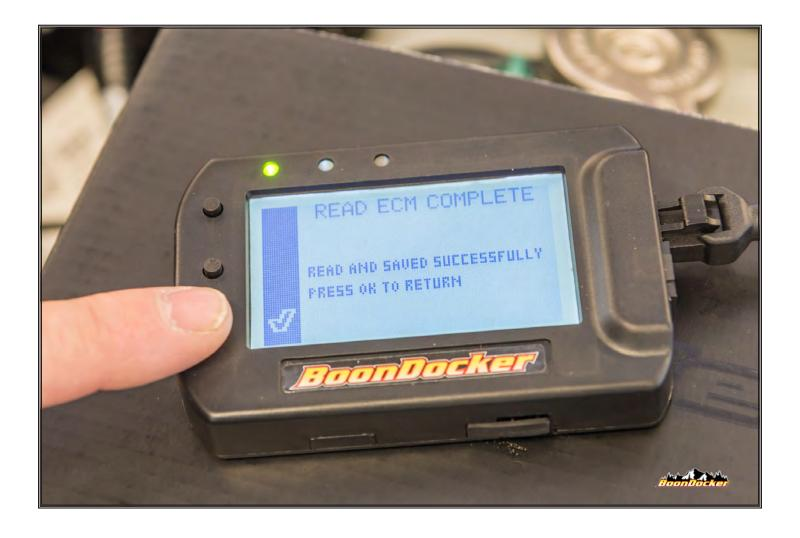
Once the ECU Read is complete, press the bottom button to return to the previous menu.
