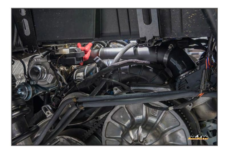
Install charge tube as shown. Verify routing of spark plug lines. Install BOV.
