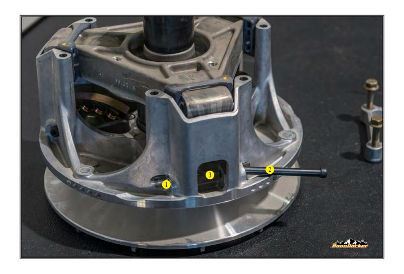
PERFORM ONE AT A TIME, FOR EACH OF THE (3) WEIGHTS: Loosen nut 1 and partially remove bolt 2 to allow removal of weight 3.
