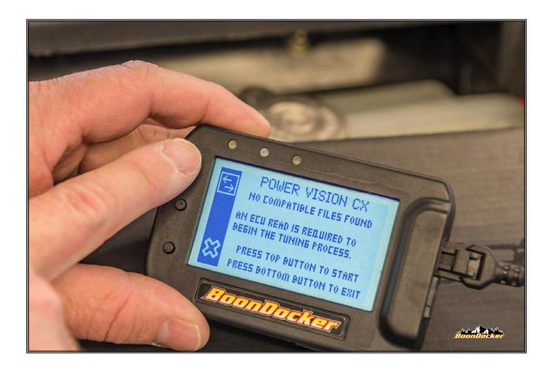
After a series of boot-up screens, you will get a message "No Compatible Files Found". Press the top button to begin reading the ECU and building the stock file.
