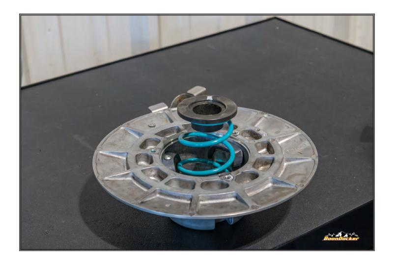
Replace secondary spring with "Teal" provided spring. Install hardware.
