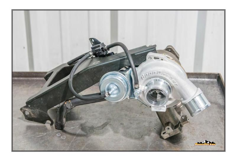
Install BoonDocker Turbo onto factory bracket as shown. Use supplied zip ties to fasten tubing around barbs on turbo and wastegate.
