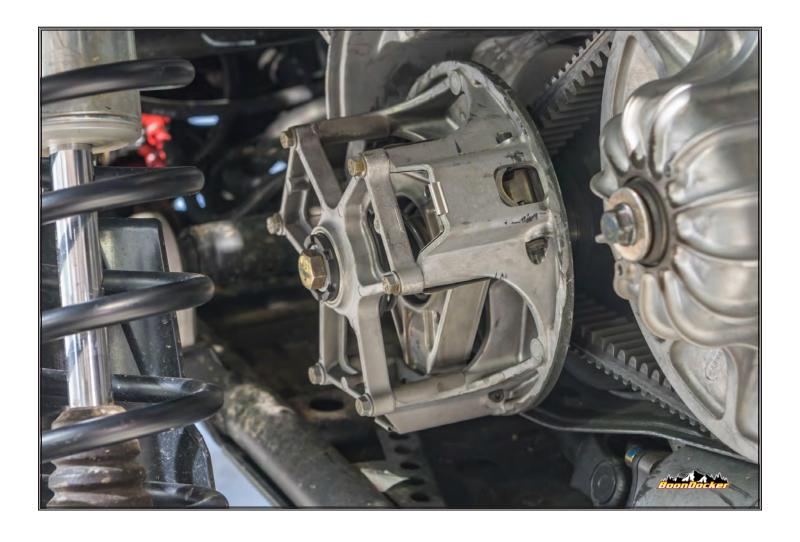
Remove primary and secondary clutches. Primary clutch WILL REQUIRE a special tool for removal.
