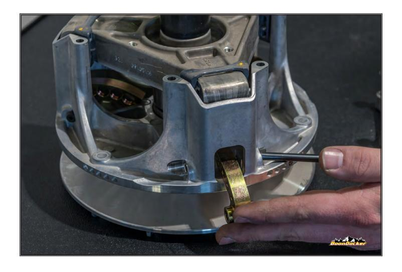
Install new weights as shown. Use original nut and bolt. Tighten to OEM spec.
