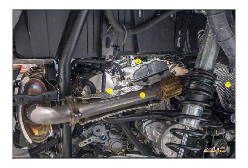
Reinstall exhaust piping 1. Reinstall factory heat shields 2.
