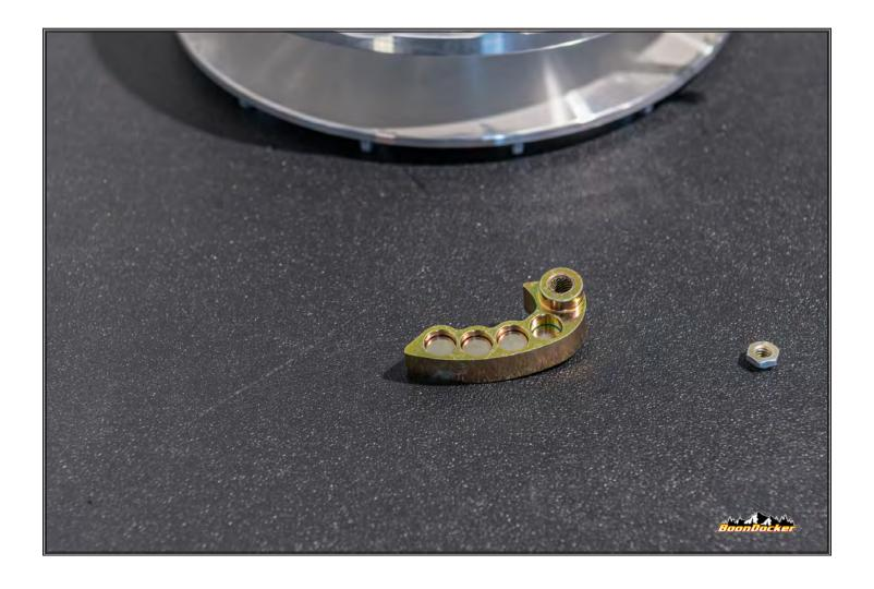
Verify placement of magnets inside of supplied weights. Weights should be loaded from BoonDocker (2-3-3-3, weights, from heel to toe)
