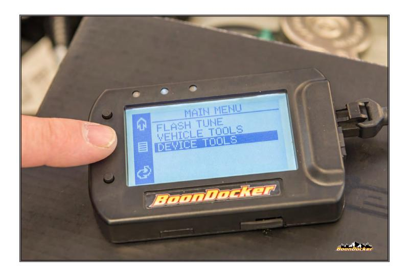
Using the buttons, scroll down to "Device Tools" and press the center button to enter that menu.
