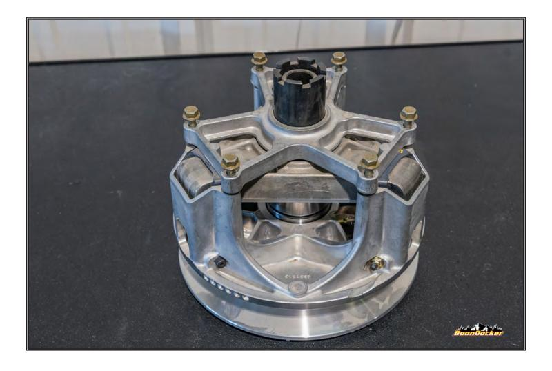
Loosen bolts to remove cover from primary clutch.
