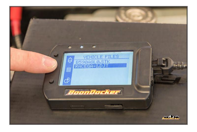
Load your Dominator tune! Use the buttons to scroll down to the tune you wish to load. Use the button to select the tune. Writing to the ECU may take 15+ minutes.
