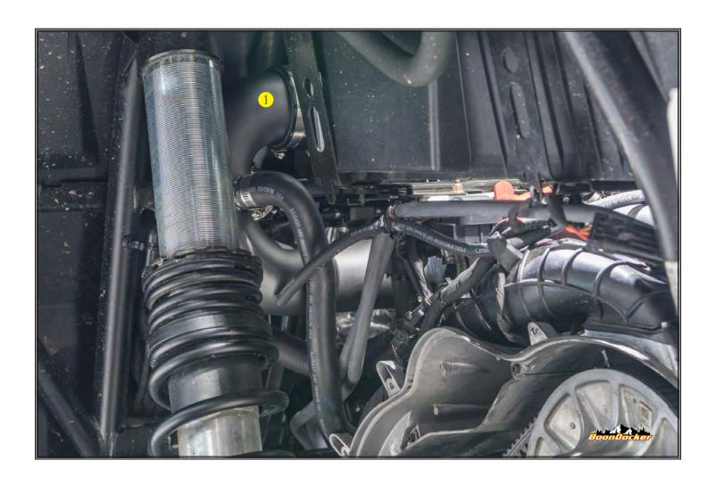
Install cold-air intake as shown ①. Tighten all hose clamps. Verify alignment, and prevent hose clamps from rubbing. Verify boost reference line is not in a bind or pinched (line not shown, but is wrapped in a nylon-webbed sheathing.
