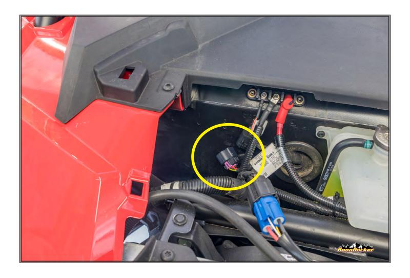
Locate the vehicle OBDI (Onboard Diagnostic Interface) port, under the hood, against the firewall. With the key in the "OFF" position, plug the PVCX Tuner into the OBDI Port. Ensure the cord is plugged into the PVCX Tuner. Once the connection is made, turn the key to the "ON" position, but do not start the vehicle.
