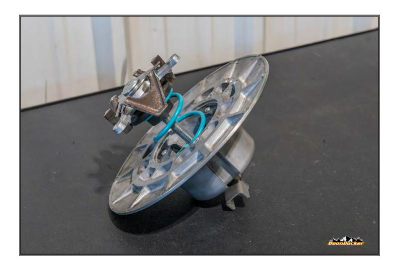
Using a clutch spring compression tool, compress the spring to allow re-installation of the (3) screws to re-assemble clutch.
