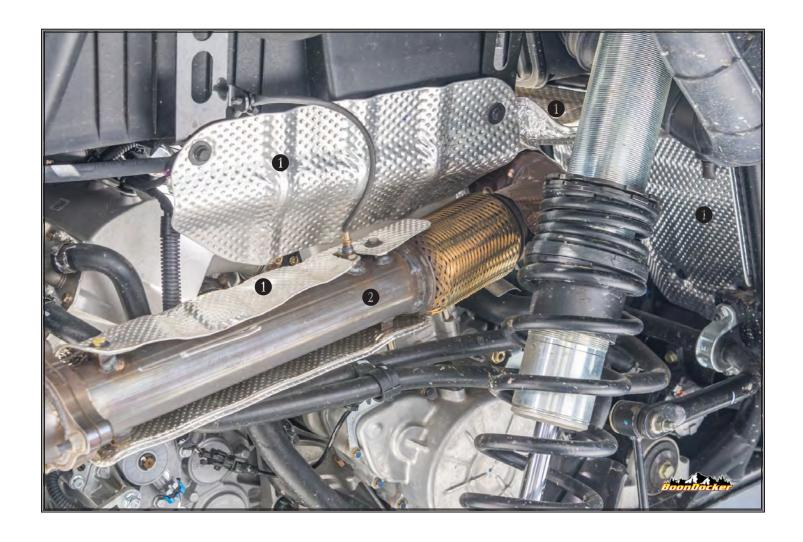
Remove aluminum heat shields ①, including the piece on top of the motor, accessed from the trunk compartment. Remove exhaust pipe ②. Muffler can be left in place.
