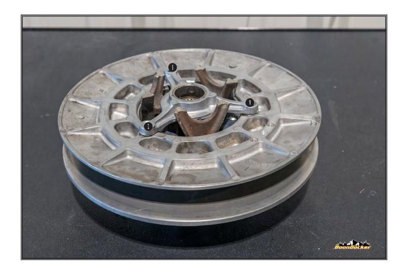
Remove (3) screws to split the sheaves 1.
