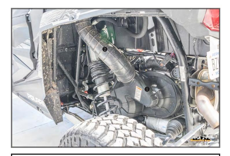
Remove plastic clutch vent 1 and clutch cover 2
