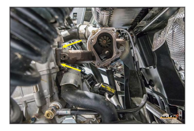
Unbolt exhaust manifold from motor. There are (4) studs with nuts, and (2) bolts. Unbolt turbo bracket from frame (easiest to access from panel behind seats/console).
