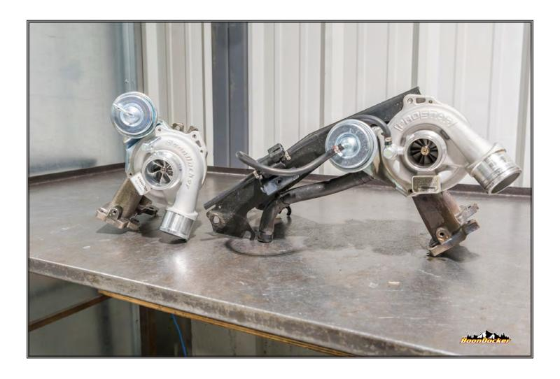
Uninstall factory turbo from bracket. Cut oetiker clamps from factory boost actuator
