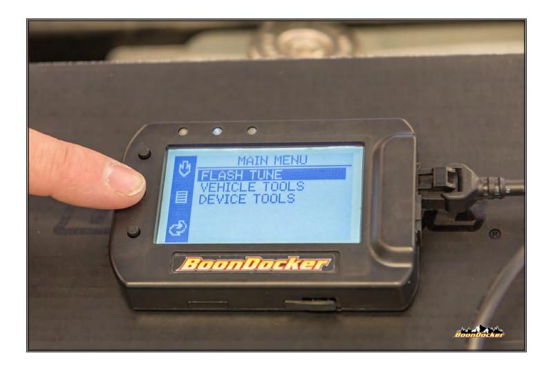
Plug the PVCX into the OBDI port as done previously. Use the buttons to select "Flash Tune"
