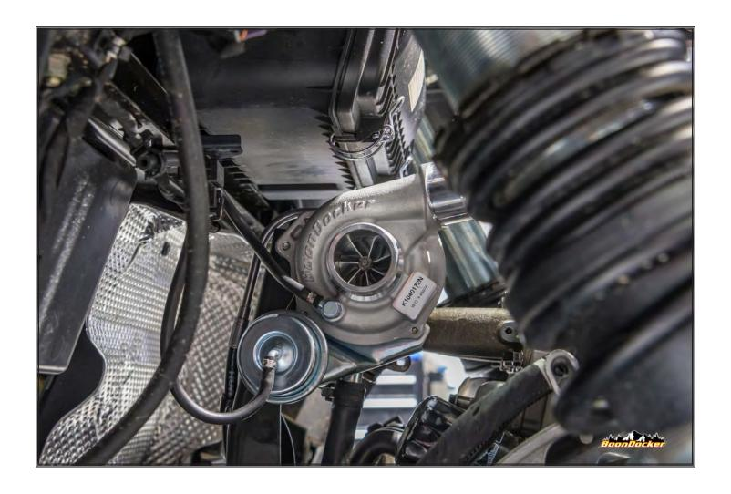
Install turbo & bracket back to car, using factory hardware. Fasten exhaust manifold to factory torque spec. Connect oil-lines to turbo. Use NEW copper gaskets for banjo fittings.
