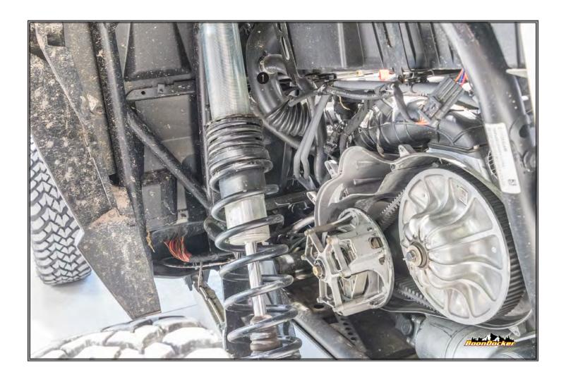
Remove cold air intake ①. Cut the oetiker clamps from cold air, charge tube, and blow-off valve (BOV)
