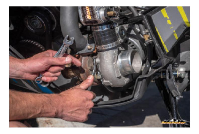
(1)Remove this bolt from the intake side of the turbo (2)Remove the outside bolt from the block off plate.
