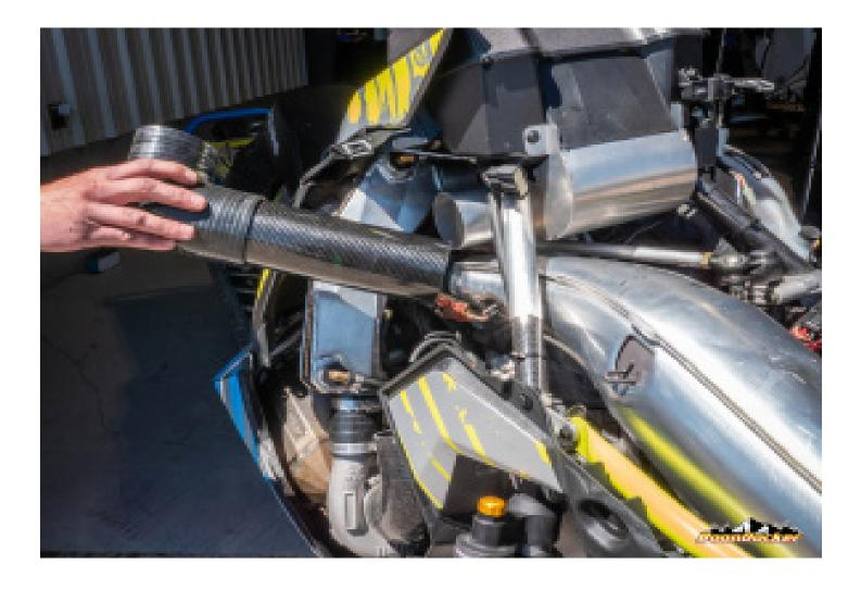
Remove cold air intake tube from the turbocharger
