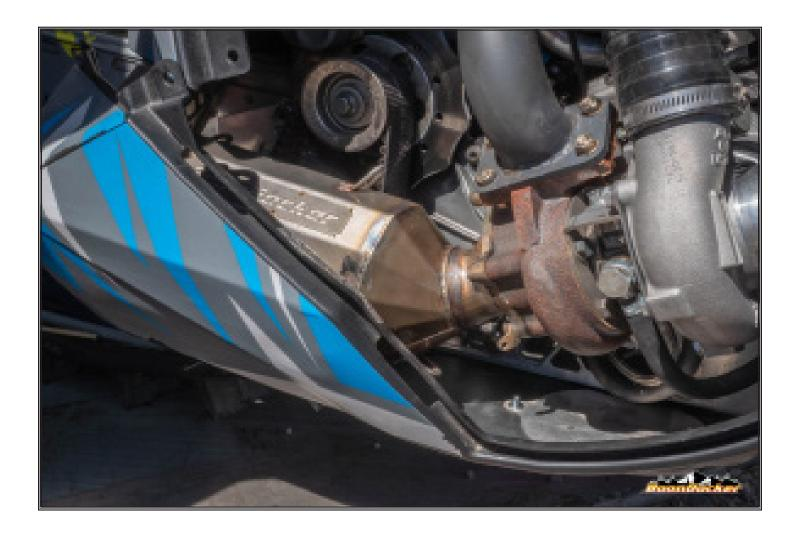
Re Install your muffler. Its easiest to put the tunnel dump side of the muffler in place, then using one hand pull on the exhaust inlet pipe towards the front of the vehicle and slide the muffler in place from the bottom up.
