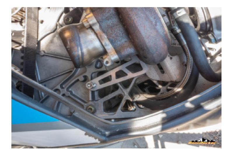
Put the bracket in place making sure that the top tab is latched ontop of the Turbo Mounting Bracket. Install the Hex head bolt into the existing threaded hole on the Chassis. Tighten ensuring the Hold Down bracket is holding the Mounting braket tight against the chassis.
