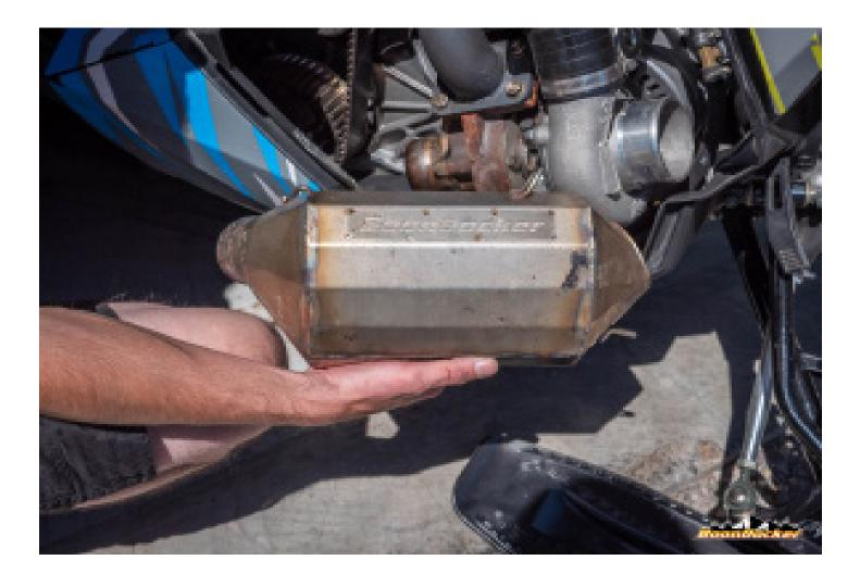
Remove the muffler from the sled.
