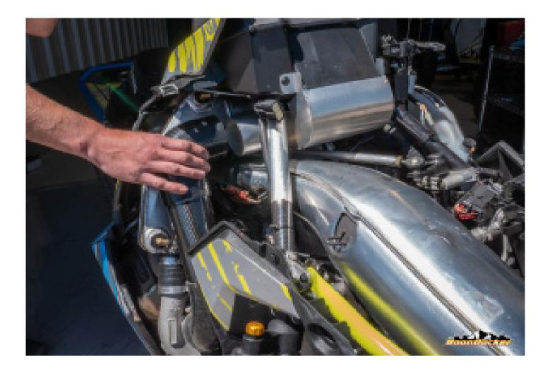
Remove the Air Intake Tube from the air box
