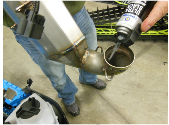
60. Use silicon on inside of flange
