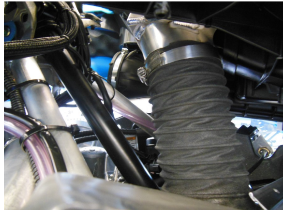
104. Set hood on sled, install cold-air intake flex hose as shown. Route intake under overstructure to turbo.
