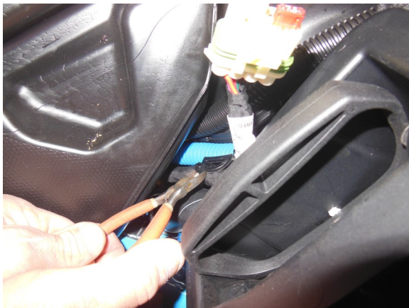
27. Cut zip-ties on the top of the air-box (mag-side) to free harness-hoses
