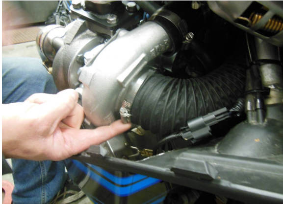
109. Connect lower side of cold-air intake tube to turbocharger. Secure with hose clamp. Note orientation.
