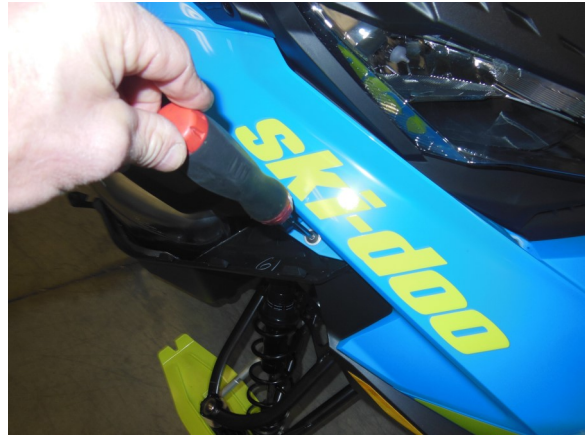
6. Remove forward small hood screws (both sides)
