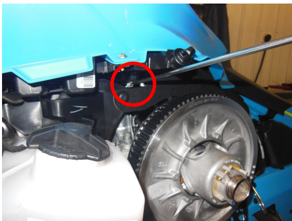
9. Disconnect factory air-intake from air-box
