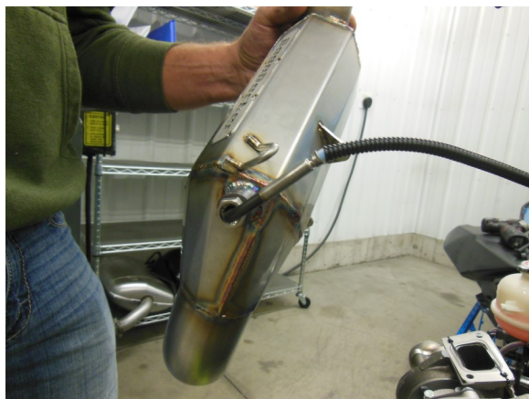
59. Install muffler temp-sensor into (new) muffler. Don't tighten, yet
