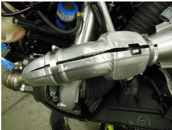
99. Re-install heat shield from pipe to turbo. Secure using supplied hose clamps
