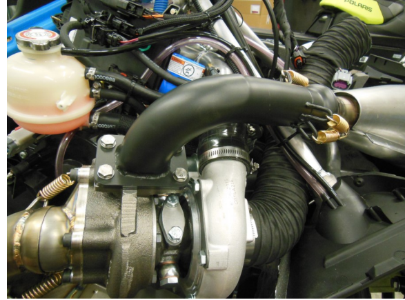
90. Install springs. Long end of spring goes towards exhaust pipe
