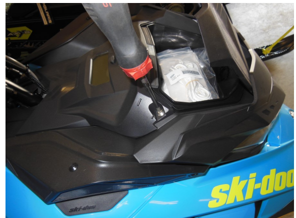
108. Plug in factory gauge and install glove compartment. Fasten using stock screws.
