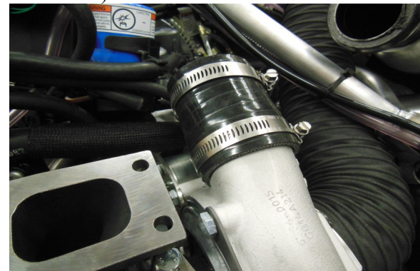
84. Install silicon hose onto turbo. Take note of clamp orientation. Tighten hose clamp on turbo-side.
