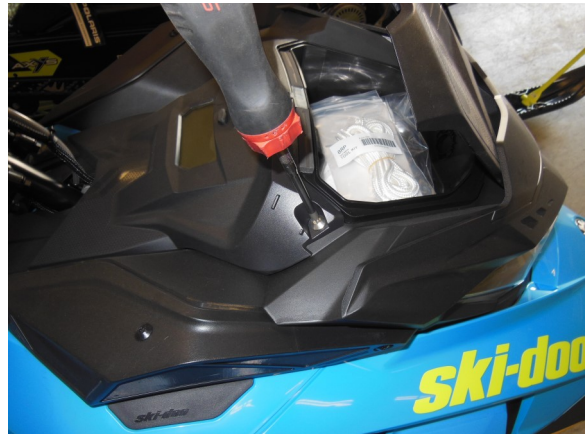
2. Remove the glove-compartment screws and remove the glove-box compartment
