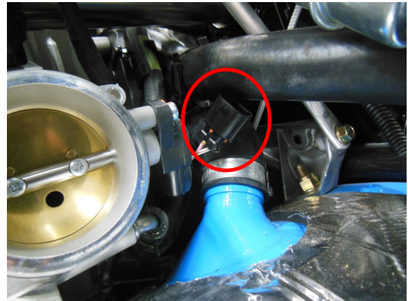
68. Disconnect factory TPS connection
