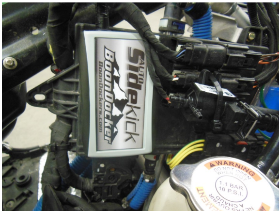
101. Clean ECU surface with rubbing alcohol. Slide control box behind factory harness as shown and attach with Velcro to ECU surface as shown.
