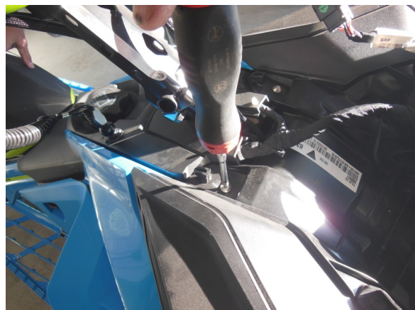
4. Remove two screws under the gauge cluster
