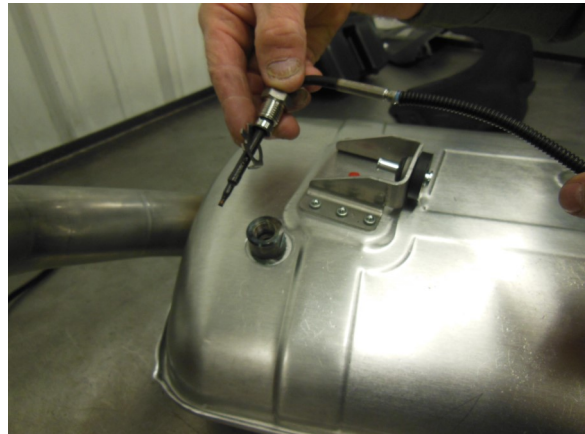
38. Bend tabs back and unbolt/remove muffer temp-sensor
