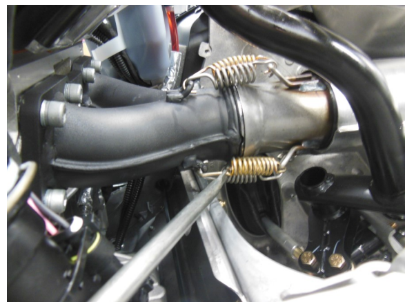
40. Double up all exhaust springs with (new) springs (Y-pipe to pipe)
