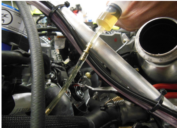
49. Fill (new) turbo oil feed line with 2-stroke oil
