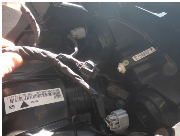
3. Disconnect hood wiring (headlights/MAP sensor/factory gauge), unplug and remove gauge
