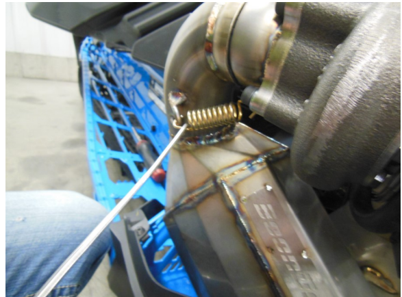
62. Install upper spring on muffler
