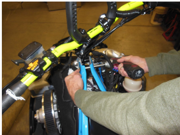
17. Remove overstructure assembly bolt where steering post connects to overstructure. DON'T DROP THE SPACER
