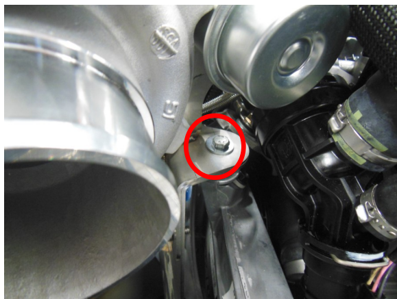
51. Install upper-turbo bracket bolt and tighten
