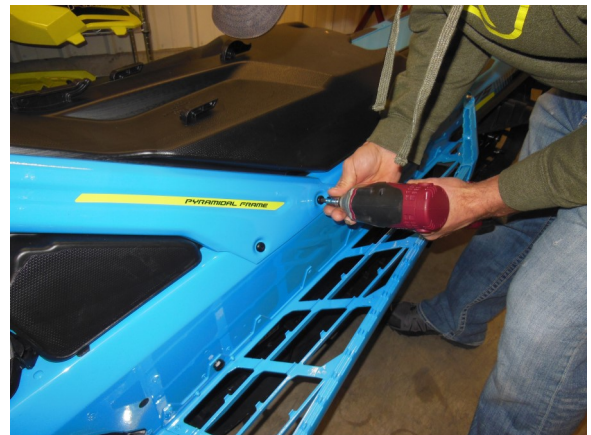
16. Remove rear screws (2 each side) from overstructure
