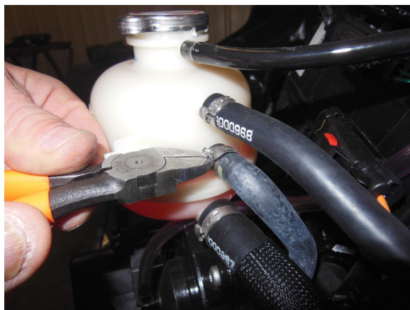
41. Cut and remove MIDDLE otiker clamp. DO NOT TWIST OR MANGLE. Don't break nipple
