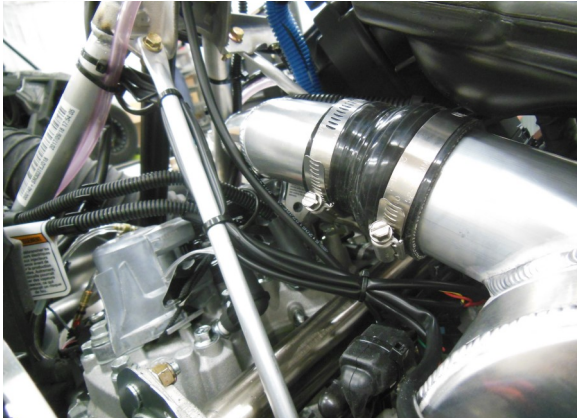
85. Install reducer on air box and aluminum boost charge tube as shown. Take note of hose clamp orientation. Tighten all connections
