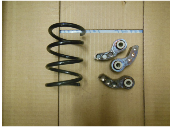
112. Install BoonDocker Supplied clutching. NOTE-Weights are already PRE-LOADED to spec.
