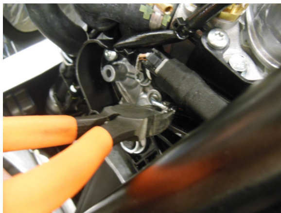
47. Cut clamps feeding exhaust valve oiling system (2 clamps, one on PTO and one on MAG side)
