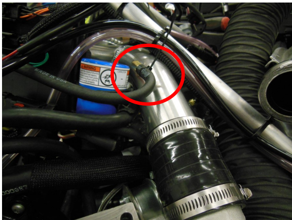
87. Install boost solenoid reference line and zip tie as shown
