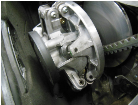
110. Remove primary clutch. You will either need specialty tools or will need to visit your local Ski-Doo dealer for assistance on installing clutching. Please refer to Ski-Doo Service Manual for proper installation technique.
