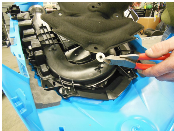
93. Move to the hood. Turn it upside down. Remove the retainer washers and sound shield
