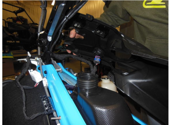
14. Cut zip-ties, unplug wire harness for tether/switches, and remove shroud.
