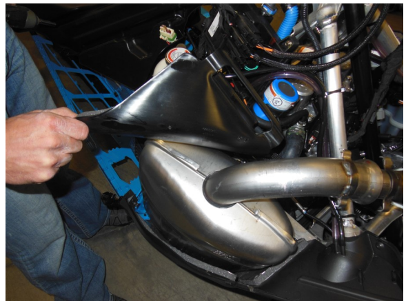
34. Remove screw from coolant bottle, and remove plastic sound-shield
