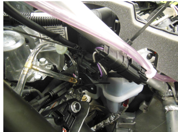
78. Install BoonDocker coil harness as shown. USE DIELECTRIC GREASE on this connection
