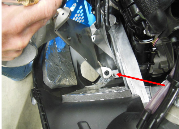
43. Install turbo/bracket by setting onto lower pins
