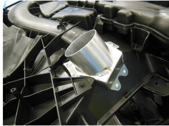
96. Install cold air adapter as shown. Carefully install screws. DO NOT STRIP.
