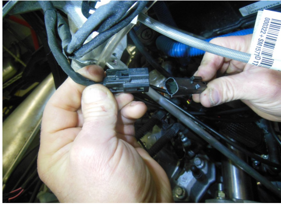
73. Plug BoonDocker harness into factory "Accessory" plugin, previously unplugged from console by hand-warmer switches
