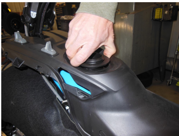
11. Remove fuel-tank jam-nut
