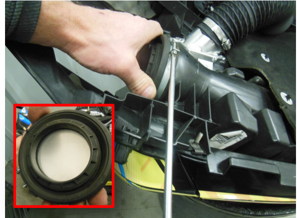
98. Install aluminum block-off plate in previously removed air-box grommet and install this assembly on factory cold-air intake.
