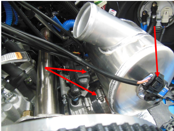
81. Install Airbox, tighten clamps, install sensor
