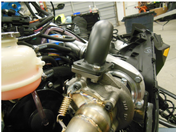
89. Install turbo inlet pipe and tighten. Don't forget the gasket
