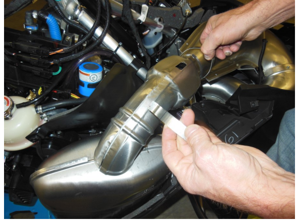
30. Remove spring-clamps from exhaust pipe heat-shield
