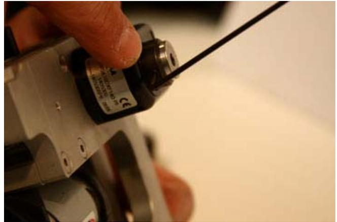
**Step 5:** With the 5mm allen key hold the center axis screw at the top completely still. With your hand slow rotate the black barrel in the direction you need to get the dial to read 90.0 again.
