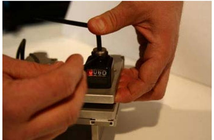
**Step 6:** Remove the set screw you installed to help you rotate the barrel
