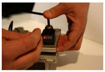
**Step 6:** Remove the set screw you installed to help you rotate the barrel
