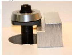
6. Use a low speed setting. You will have to experiment with the speed setting as all routers differ in their speed settings. You do not need a very fast speed. Typically with 1½ horsepower router a setting of "2" is sufficient.
