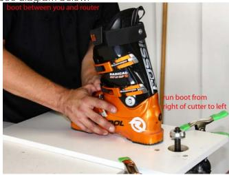
Note - Failing to run the boot against the rotation of the cutter will result in a sudden impact and can shoot the boot from your hands possibly causing personal injury and/or damage to the boot.
