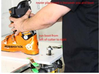
If you run the boot in between you and the router placement – you run the boot from right to left. See diagram below.
