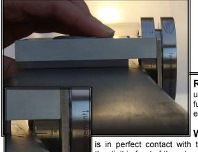
Rotate the disk until the pawn fully tangent the edge
