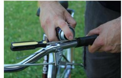
Clean the bar thoroughly with alcohol or soapy water to remove any residue. Use a scouring pad or extra fine steel wool if the residue warrants.
