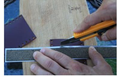
You will need a straight edge, utility knife (with a new blade) and a cutting board. Place the grip finished (coloured) side up on the board. Place the straight edge equal distance between the pair of holes on either side of the grip closest to the desired measurement. (If possible leave an even number of holes on each side. This makes lacing slightly easier.)
