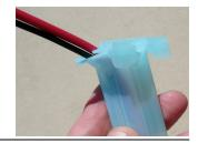
The photo on the right shows a typical connection when small gauge wires have to be connected. Note the loop of 14 AWG wire used to facilitate the insertion into the gel-filled tube.
