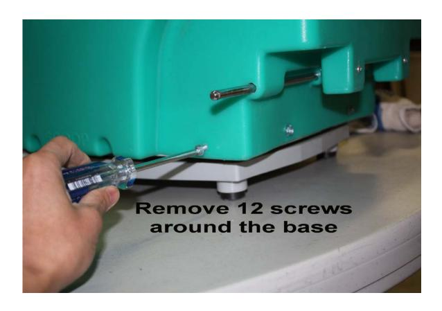
B.REMOVE THE SHELL FOR REPLACING MOTORS OR WHEELS
