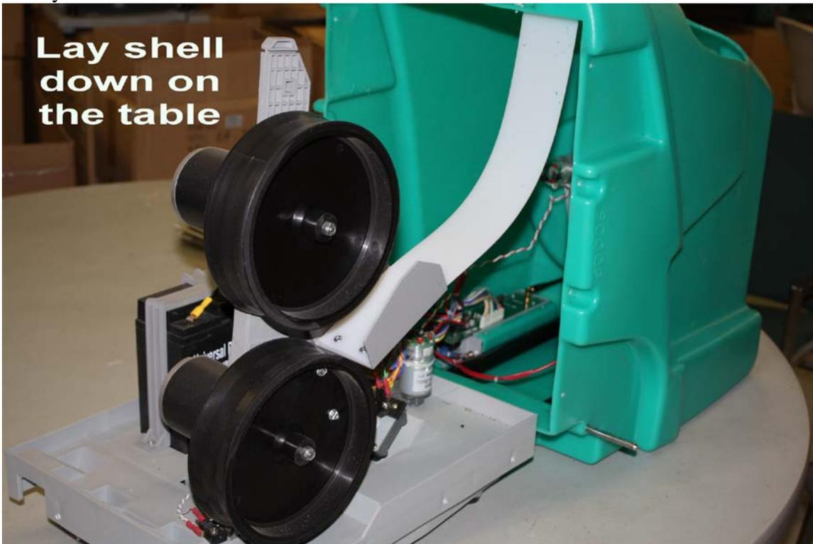
F. Disconnect feed motor's wires if it is too tighten
