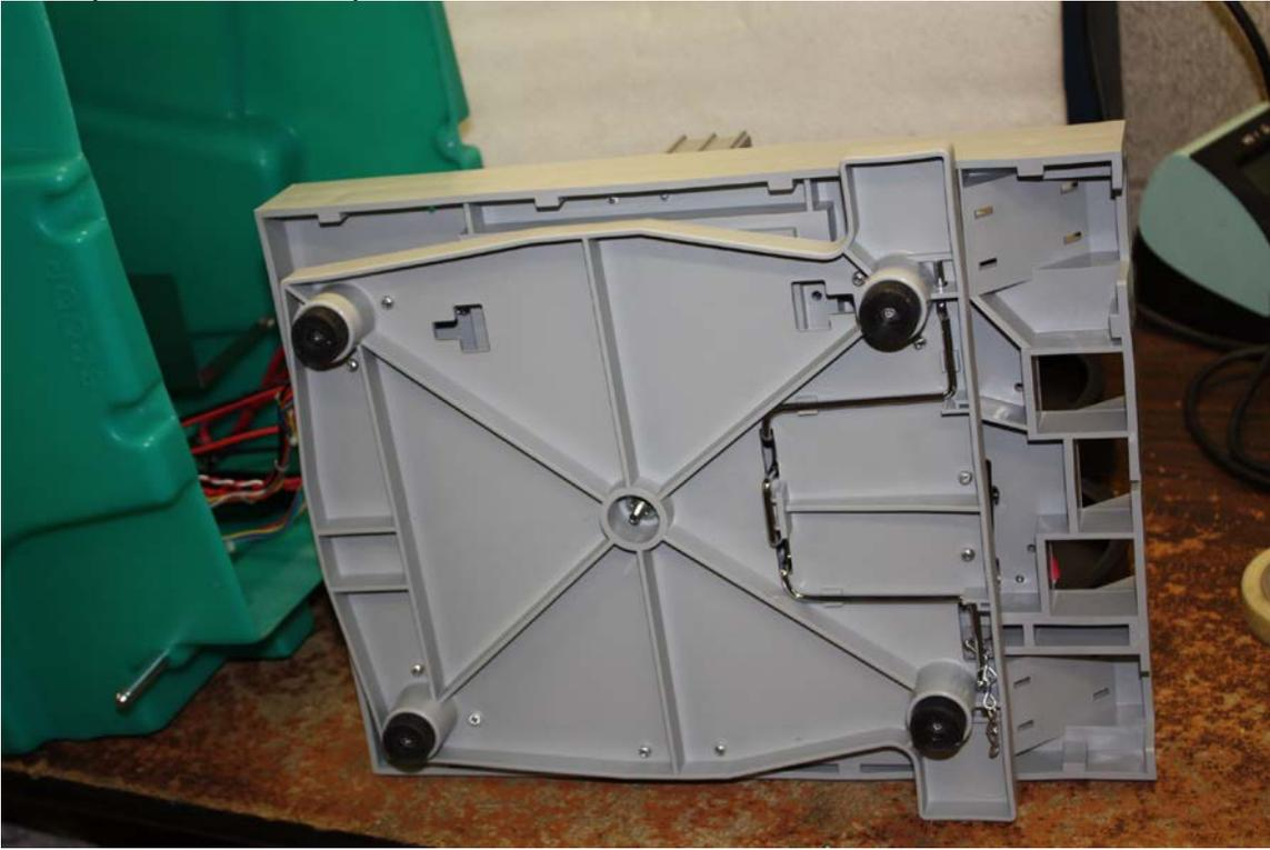
I. Remove 2 screws and nuts for fixing battery holder
