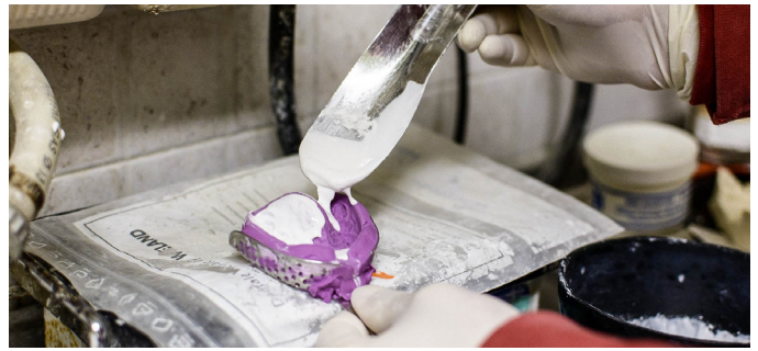
After receiving a dental impression from a dentist, OpLab used to create a plaster cast.
