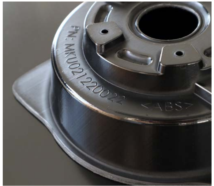
Automotive prototype part made on the Mayku Multiplier.
