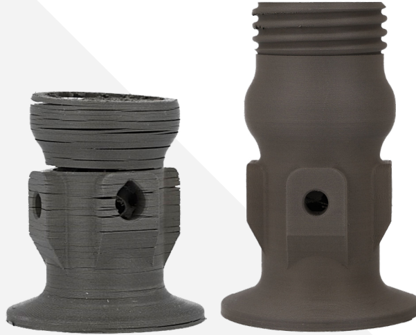
Figure 19. Cooling & Delamination example
