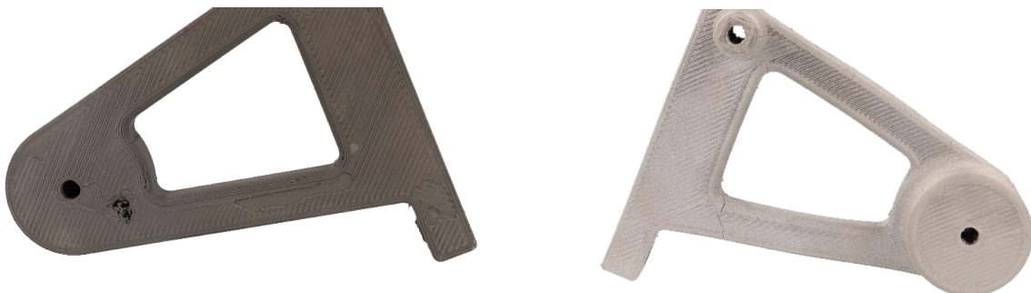
Figure 18. Damaged Bottom surface & resulting top cracks
