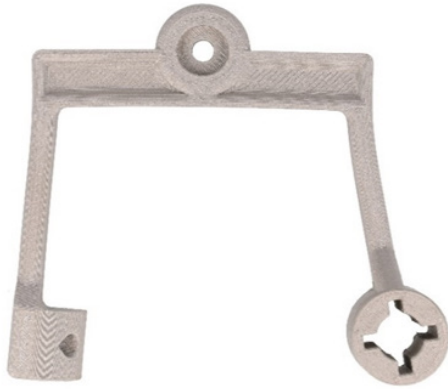
Figure 21. Part with distortions after D&S
