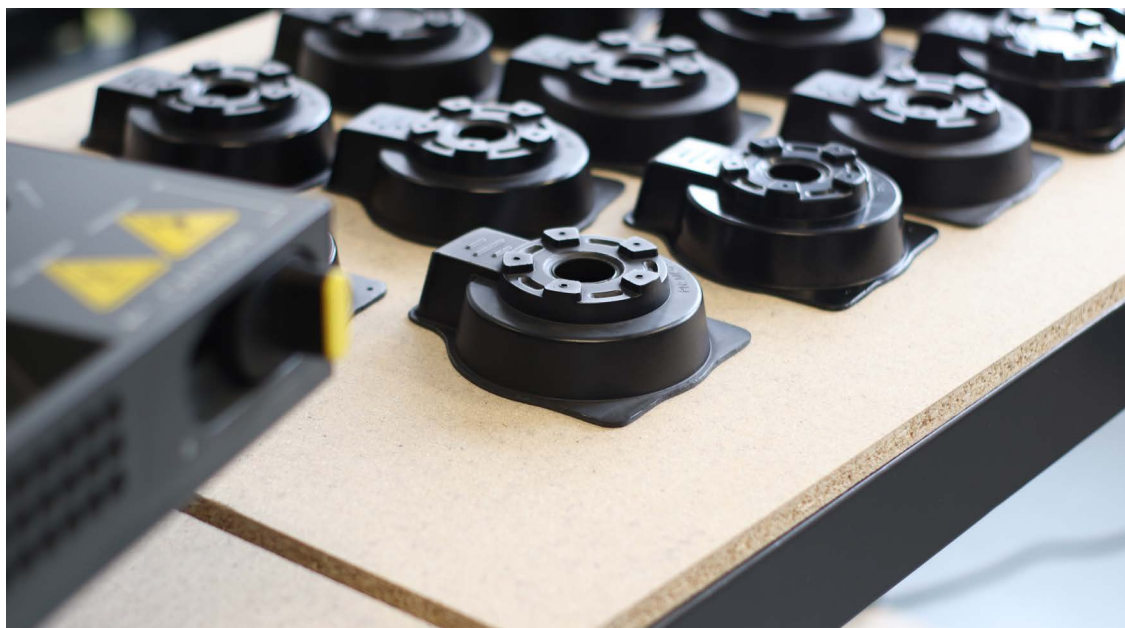
Batch of 4mm ABS parts made with the Mayku Multiplier
