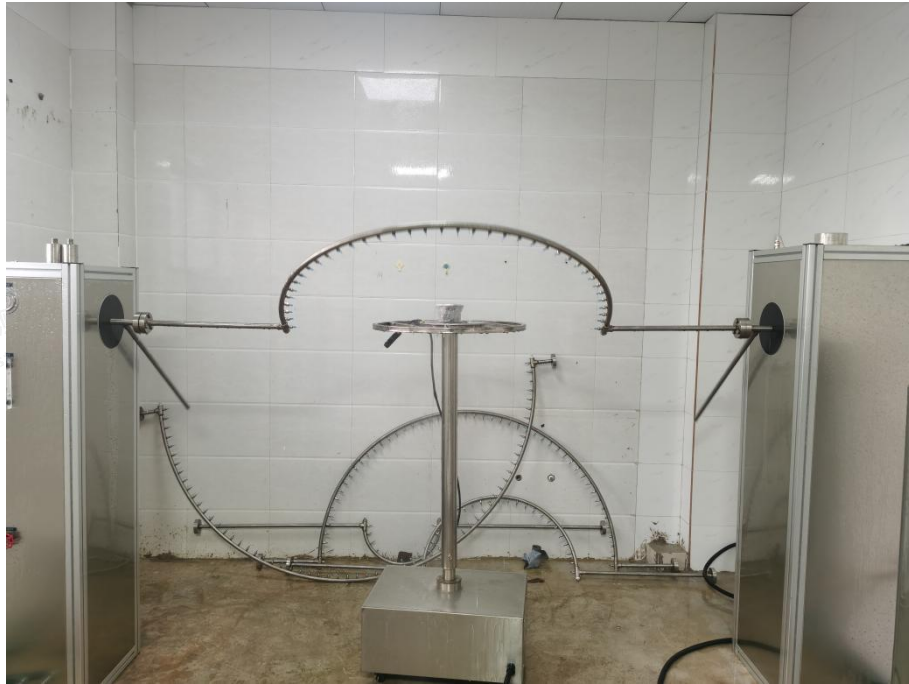
Photo 9: IPX4 test of model SOP-2ZNC
