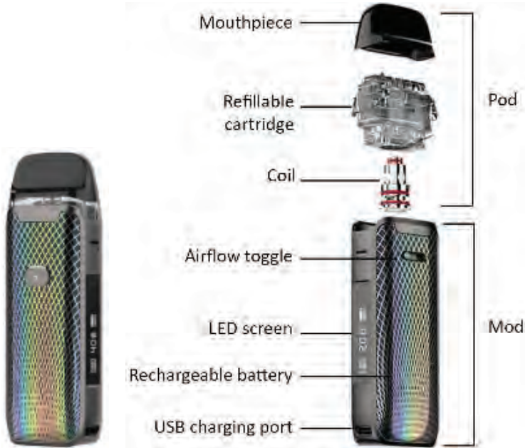
Parts of a pod mod
