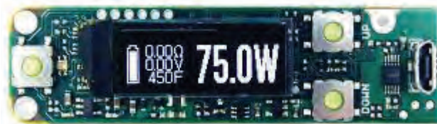
Printed circuit board with a chipset and display screen for a box mod
