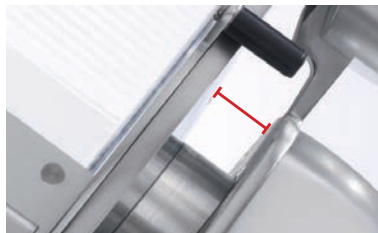
Increased gap between blade and machine body
