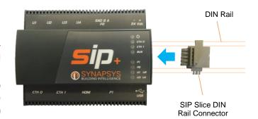
2. Slide the DIN Rail connector until it fits securely in to the DIN Rail connector mounted to the rear of the Master units.
