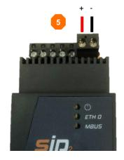
Use the MBUS with 2-pin 2-part terminal connector for a direct M-Bus metering network connection.
