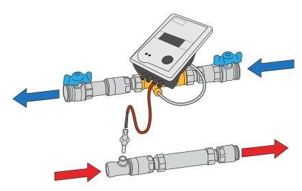
Standard version for installation on the return pipe.
