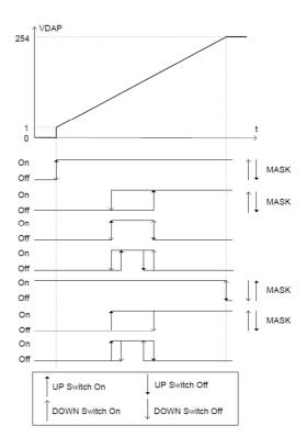
With the help of the fade time switch on and switch off delays can be realized.
