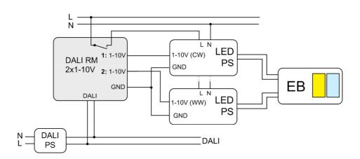
typical structure: control of two 1-10V LED-power supplies (one for CW, one for WW)
