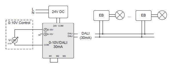
typical application with 0-10V voltage on input P (input passive, 0-10V control = source)
