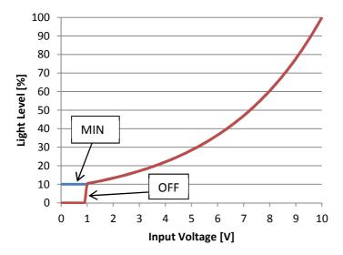
The light level is the ouput power of a standard DALI-ballast (IEC62386-102) which is connected to the converter.
