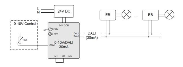
typical application with 100k potentiometer on input A (input active, 0-10V control = sink)
