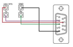
Connection diagram of a cable from RJ45 -> SubD (for direct connection to the RS232 of a PC, supply via RTS-Pin):
