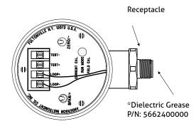
Field Wireable Connector P/N: 42119B0000 (without cable)
