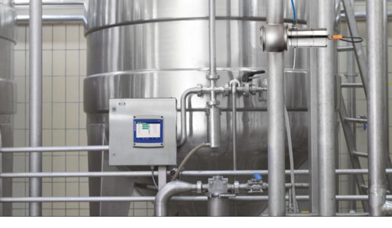
InPro 5500i: The single-piece membrane cap has been designed for fast, simple replacement and high cleanability-in-place to prevent contamination. The sensor is available with Tuchenhagen Varinline, TriClamp, and 28 mm M42 process connections.
