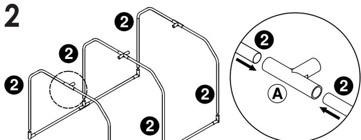
**IMPORTANT:** Push tubes into plastic connectors completely. Failure to do so may cause cover to rip.
