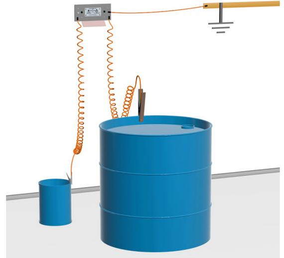
To remove static electricity from the EX/HAZLOC atmosphere grounding clamps should be capable of achieving connections to equipment with resistance values that do not exceed 10 ohms.
