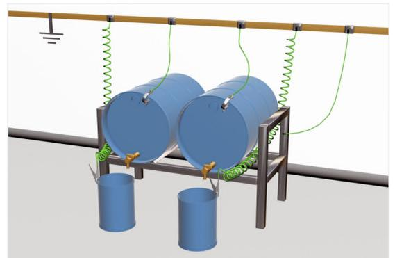
**Cen-Stat™** Static Grounding clamps, cables and reels
