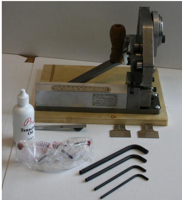
Basic Components of the Spoke Cutting & Threading Machine
