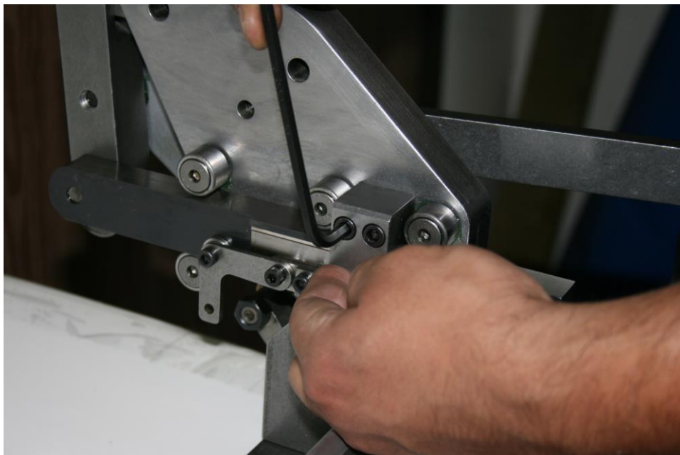
Tightening the slide support bolts
