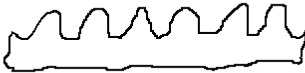
Comparison of good spoke threads and those formed on worn dies
