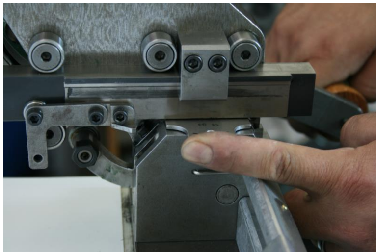
Remove the spacer to avoid jamming it against the dies when the crank is returned to it's starting position
