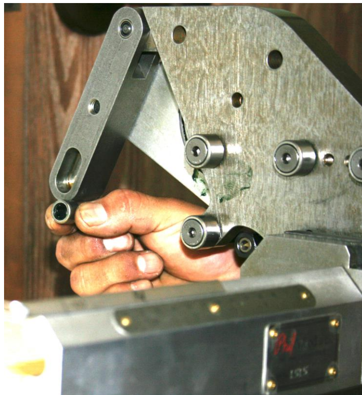
Bearing in swing slot
