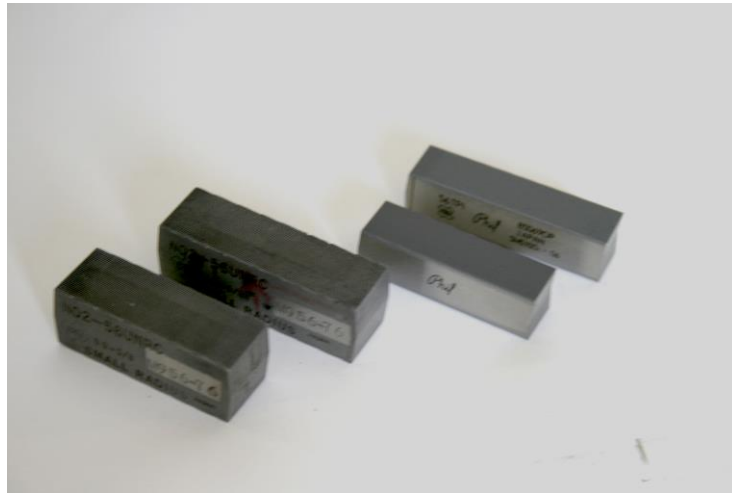
Left: Die set for machines numbered up to 188 Right: Die set for machines numbered 189 and up
