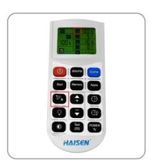
b. After entering the setting mode. Press the same button according to the icon displayed on the right side of the screen, as shown in the picture. When the icon ""on the screen flashes, you can press the ""o" two buttons to adjust the parameters. The remaining four functions ""o" on the same operation. Click the same button (the icon on the screen will flash), then press the ""o" button to adjust the parameters.
