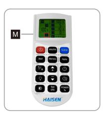
C. After the function setting is completed, press "button and the "M" icon will appear on the screen, then press "button to complete the setting.
