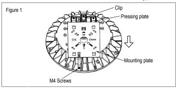
3.Connect the clip on the fixture to the spindle of the mounting plate to make sure the fixture will not slip and fall.connect the line voltage to the wires coming out from the fixture following the wiring diagram. Push the pressing plate into the suspension loop on the mounting plate.
