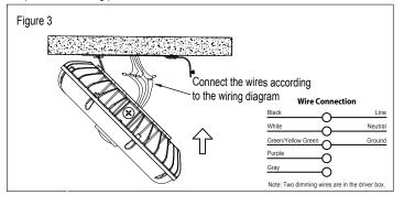
2. Fix the mounting plate to the ceiling with the screws.
