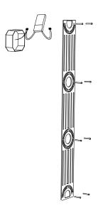
Connect fixture to LED driver, the white wire is negative (-) and the black wire is ositive, then with the provided screws secure the fixture to the already installed t-bar.
