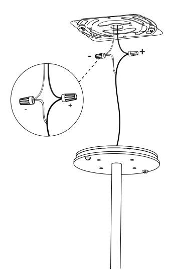
Using provided screws, install the fixture to the universal cross bar.
