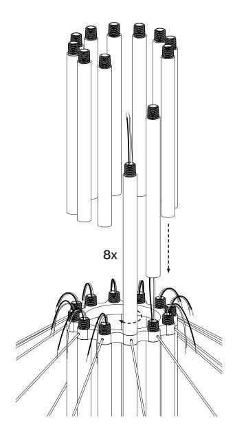
Insert the canopy on top of the stems and lock it in place using the provided hex nuts.
