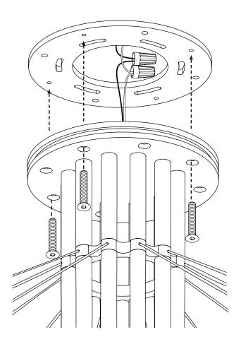
Install the glass globes by unscrewing the retaining rings and carefully slide the globes in place. Screw back the retaining rings firmly.
